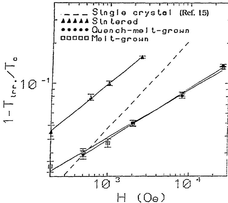
Fig. 2. Irreversibility temperature ( $T_{irr}$ ) plotted as  $1 - T_{irr}/T_c$  vs. magnetic field ( $H$ ) for melt-grown, quench-melt-grown, and sintered YBCO samples. Dashed line represents single-crystal data from Ref. 15.
