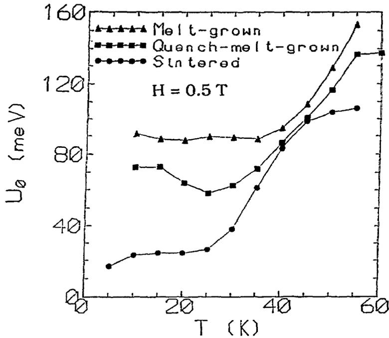
Fig. 1. Temperature dependence of apparent pinning potential ( $U_0$ ) for melt-grown, quench-melt-grown, and sintered YBCO.
