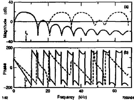
Figure 3. Frequency responses in (a) magnitude and (b) phase. Solid lines show the  $n=1$  case and dashed lines the  $n=4$  case, as determined by the Fourier transform of the coefficients. In the simulation, the phase response is  $90^\circ$  at the synchrotron frequency for both cases, due to the delays in the hold buffer.
