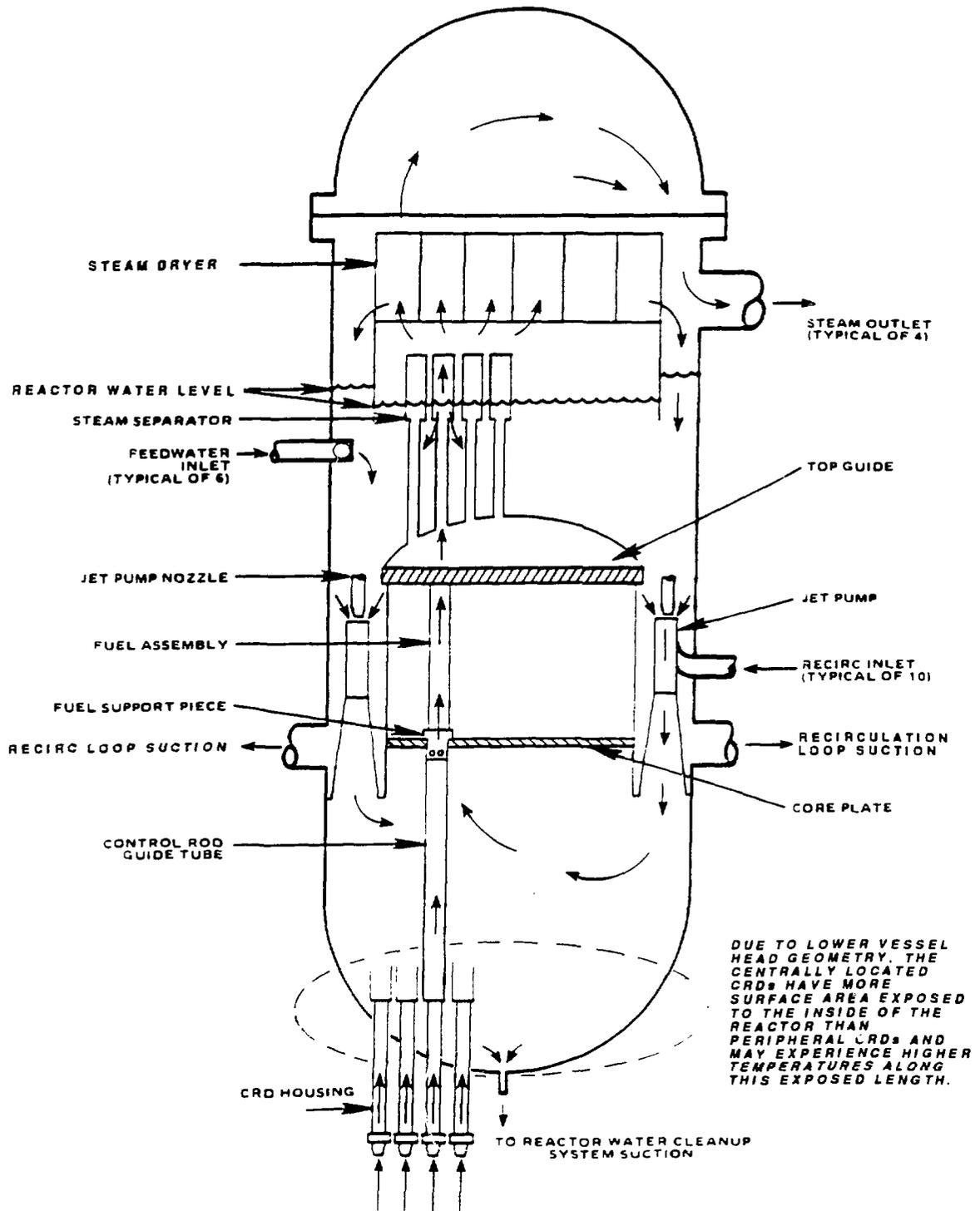
Figure 2. CRDM locations with respect to BWR lower vessel head geometry.
