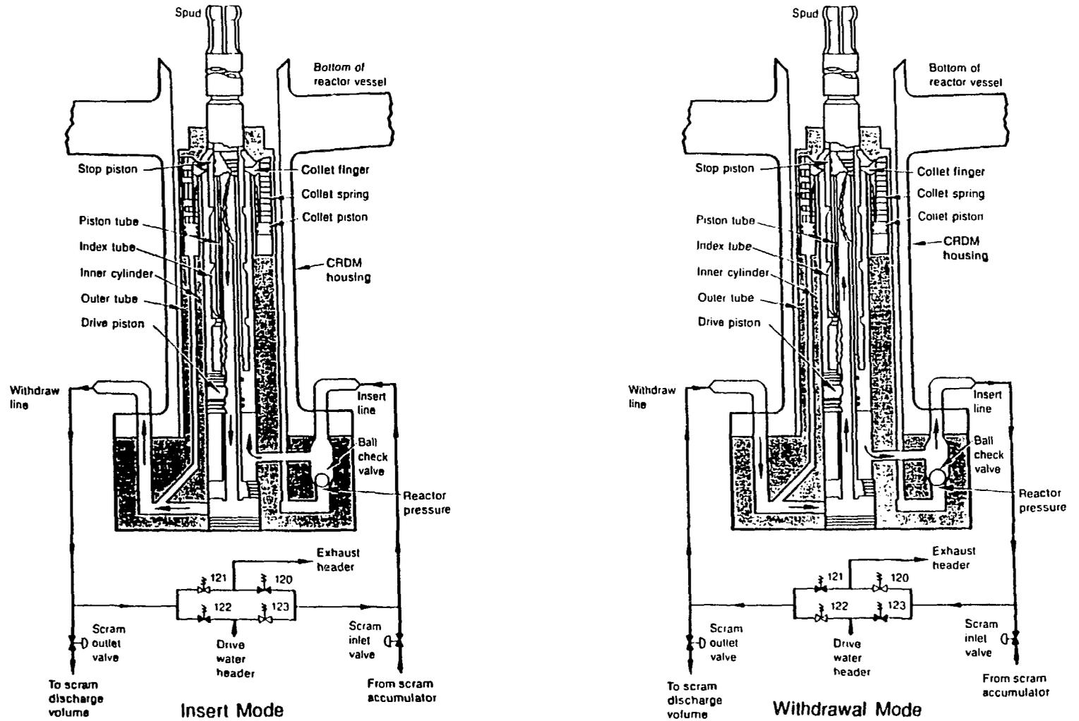
Figure 1. CRDM operation: insert and withdrawal modes.<sup>1</sup>
