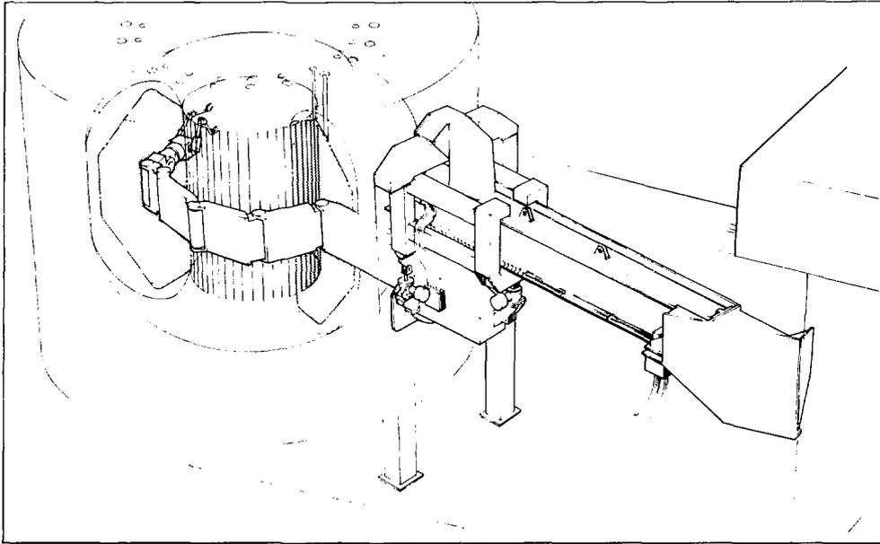
*Remote maintenance manipulator concept for Compact Ignition Tokamak. Courtesy of SPAR Aerospace.*
