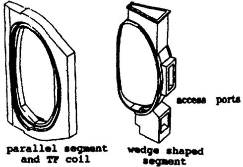
FIGURE 3: VACUUM CHAMBER SEGMENTS
