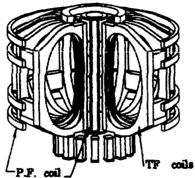
FIGURE 2: MAGNET SYSTEM ASSEMBLY
