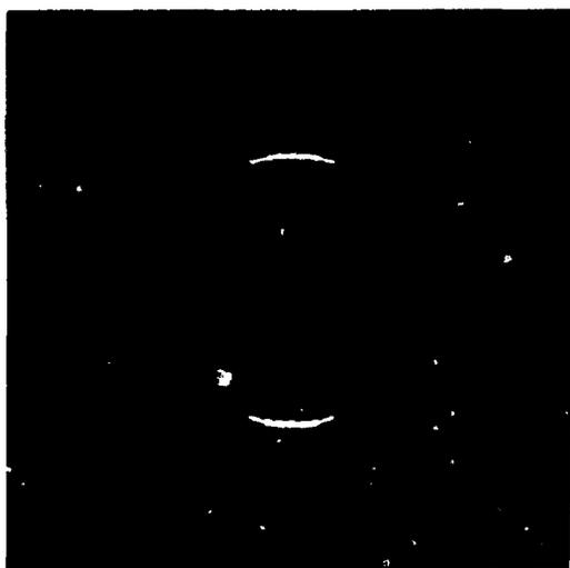
Fig. 6. Diffraction pattern from the projected potential of Fig. 2a, but for a crystal thickness of 100 Å.  $z$ -defocussing results in lost intensity, cf. Fig. 2b.
