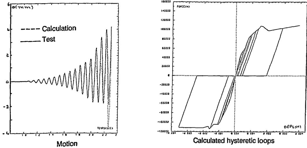
Figure 5 - Response of the wall (frequency of excitation = 13 Hz)
