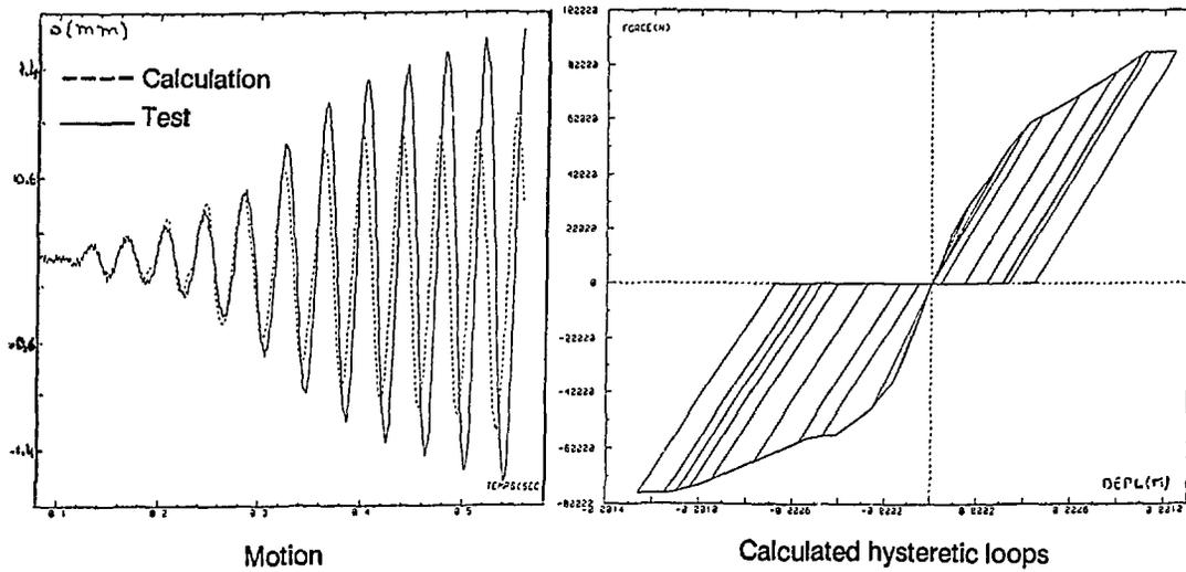
Figure 6 - Response of the wall (frequency of excitation = 26 Hz)
