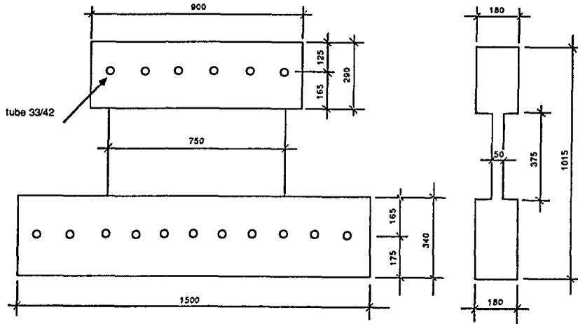
Figure 1 - Geometry of the shear wall (unit = mm)
