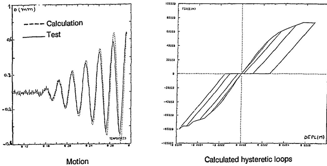
Figure 7 - Response of the wall (frequency of excitation = 40 Hz)
