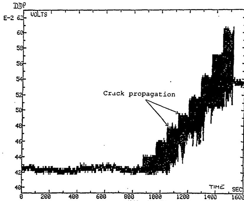
Figure 5 Typical cutted-wire gage output signal
