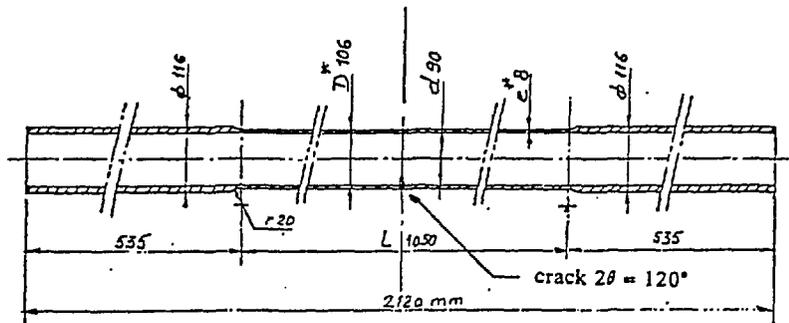
Geometrical characteristics of a pipe
