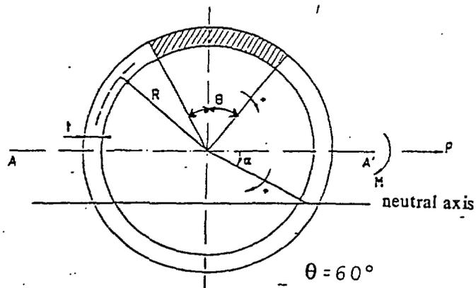
FIGURE 2 : Geometry of a cracked pipe section
