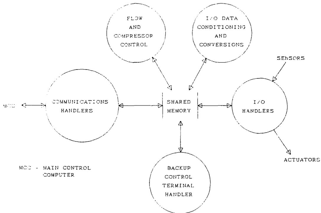
Figure 3. Main Loop Computer Simplified Software Function Diagram
