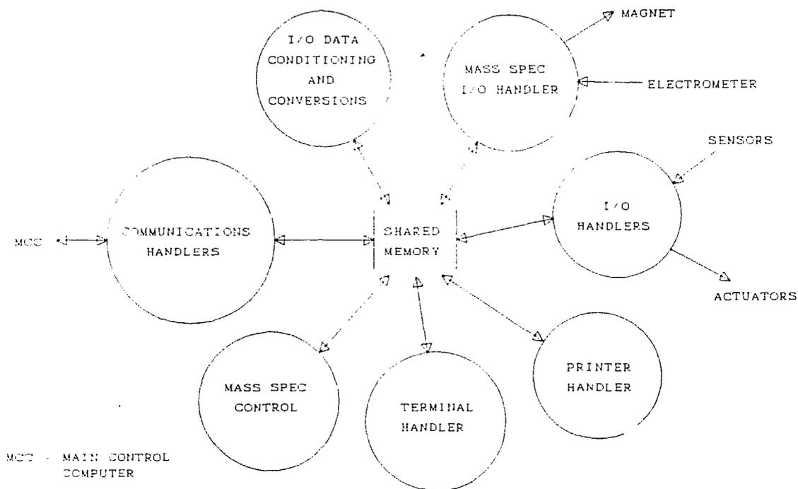
Figure 4. Tag System Computer Simplified Software Function Diagram
