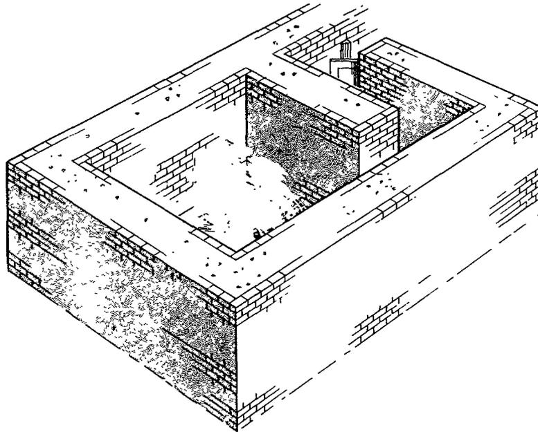
*FIG. 6. Labyrinth entrance for a walled enclosure used for shielded storage.*
