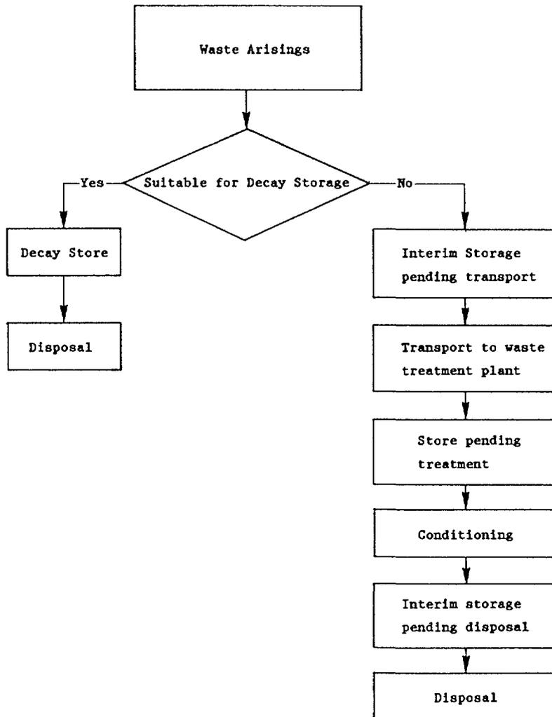
FIG. 1. Simplified flow chart showing the use of storage in the waste management system.
