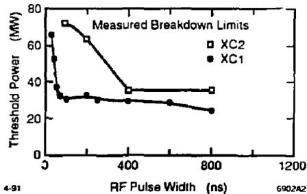
Figure 2. Performance of the first SLAC X-Band klystrons.
