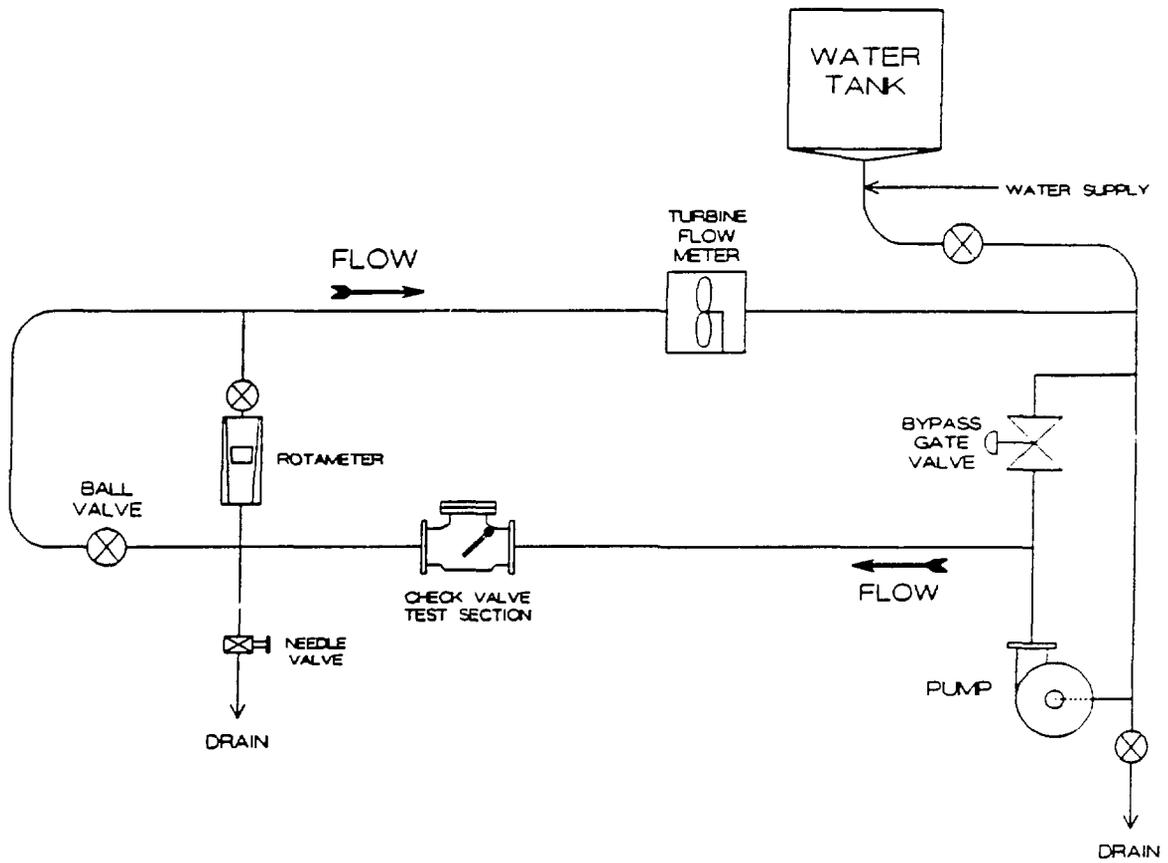
Figure 9 ORNL check valve flow loop (schematic).
