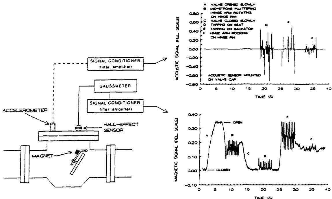
Figure 20 Magnetic flux and acoustic signatures for a check valve under several simulated operational conditions.
