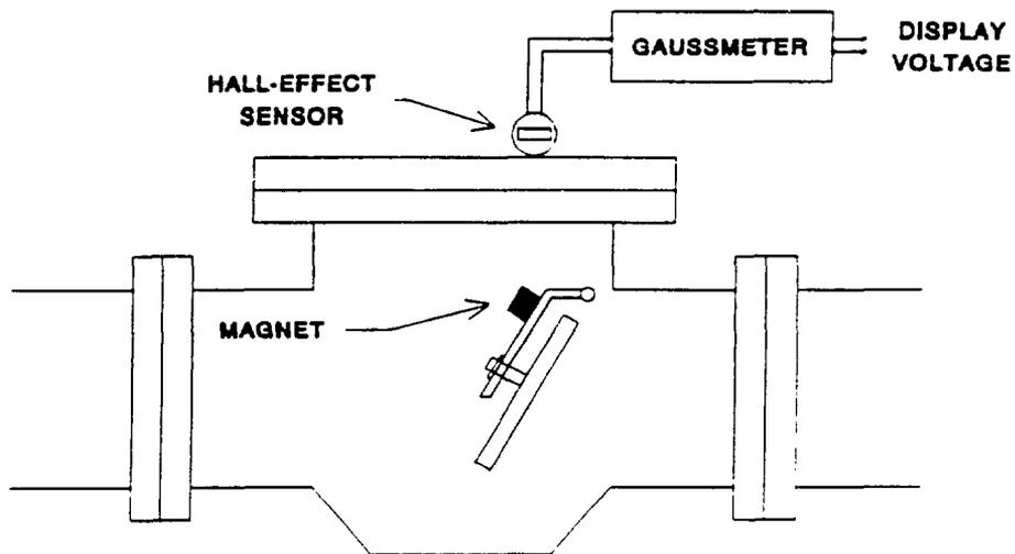
Figure 7 A simplified depiction of the magnetic flux signature analysis (MFSA) technique.
