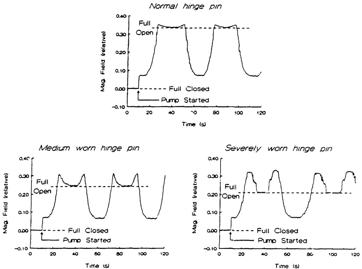
Figure 12 Magnetic flux signatures of a 3-inch swing check valve for three hinge pin conditions.
