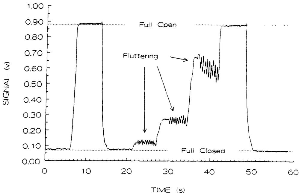
Figure 16 Application of the external DC magnet method to monitor disc position and motion of a 10-in. check valve at Oak Ridge.
