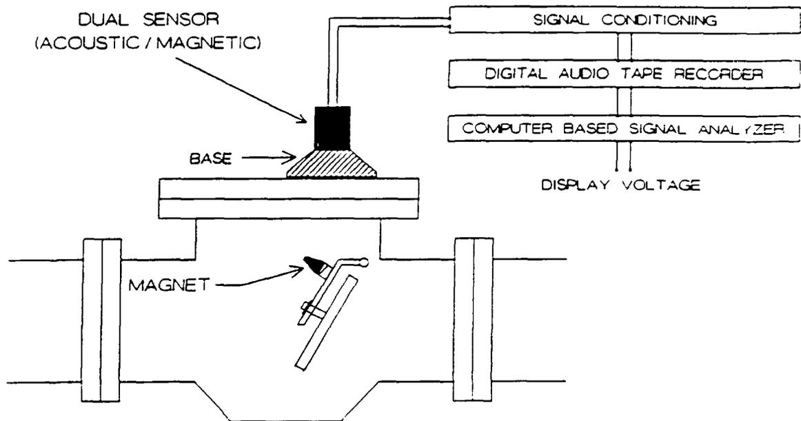
Figure 21 A simplified depiction of the dual sensor used by the QUICKCHECK™ system available from Liberty Technologies, Inc.
