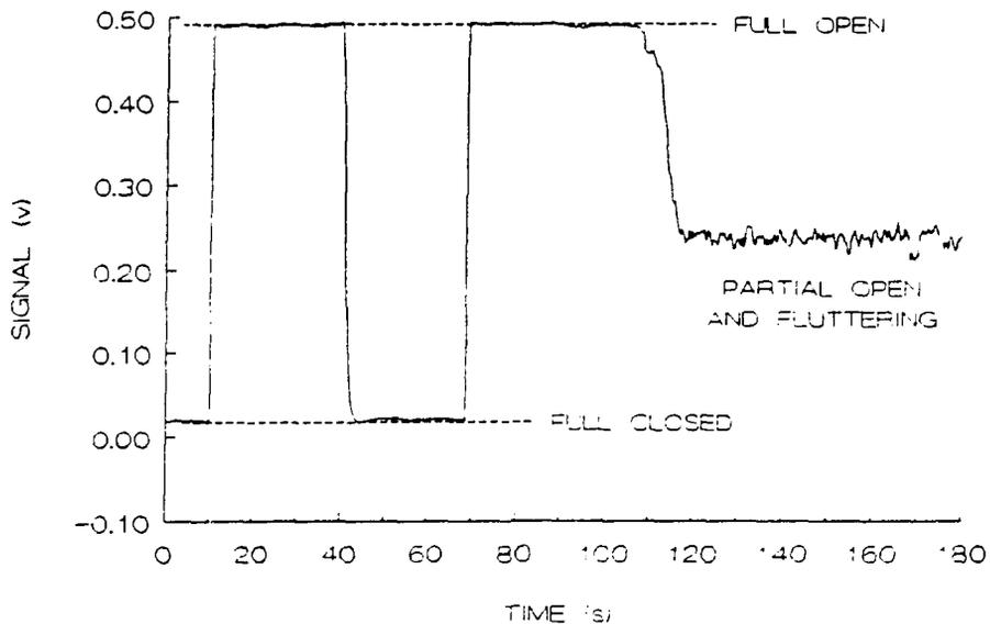
Figure 14 Application of the external AC magnet method to monitor disc position and motion of a 3-in. check valve installed in a flow loop at Oak Ridge.
