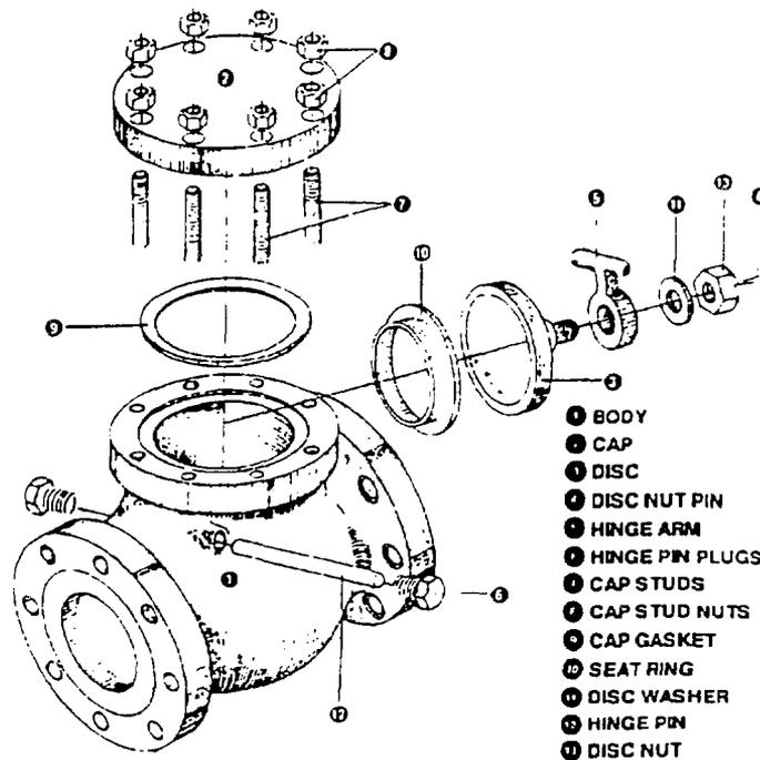
Figure 1 Typical swing check valve.
