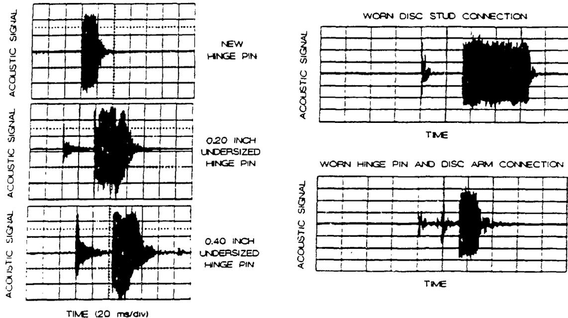
Figure 4 Check valve closures with new and artificially worn hinge pins and with worn disc stud connection. Data acquired by Duke Power Company.
