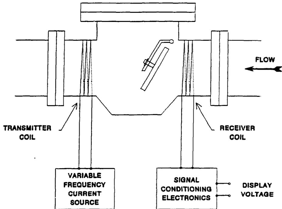
Figure 13 Simplified depiction of the external AC magnet check valve monitoring method developed by ORNL.
