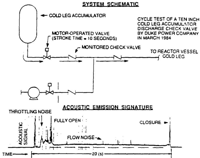
Figure 2 Acoustic signal vs. time for a 10-in. check valve tested by Duke Power Company in March 1984.
