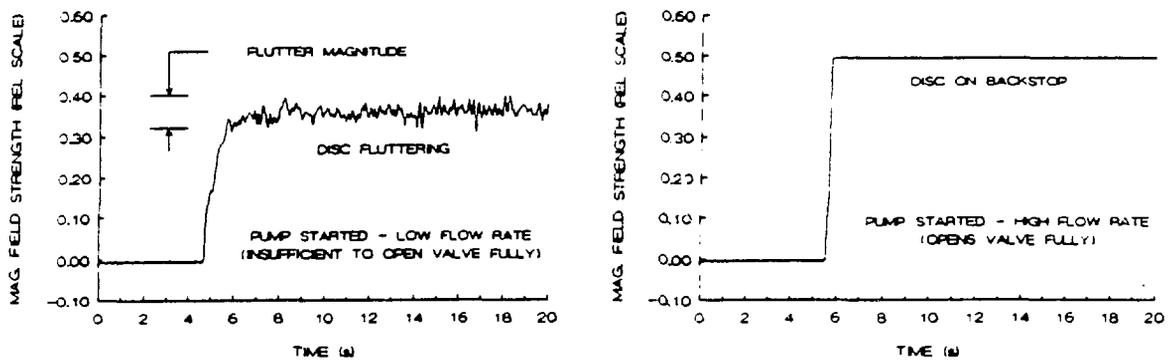
Figure 10 Use of MFSA to detect disc instability (flutter).
