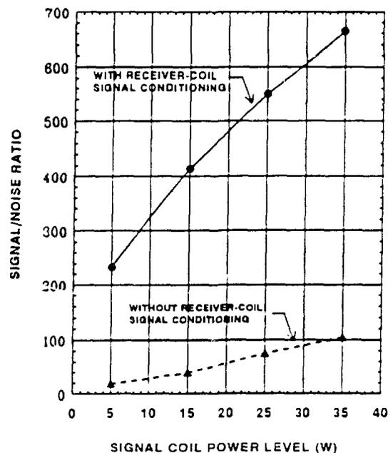
Figure 19 Improvement in signal-to-noise level observed on the AC magnetic system as a result of using signal conditioning.
