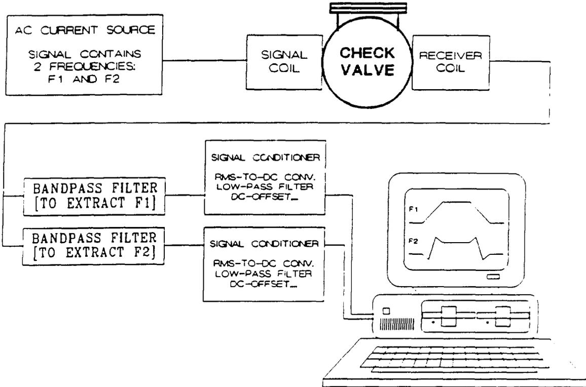
Figure 18 Illustration of a check valve monitoring system that uses two frequencies to generate two output diagnostic signals (linear and "humpback") simultaneously.
