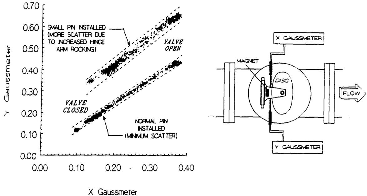
Figure 11 MFSA technique for detecting worn hinge pins.
