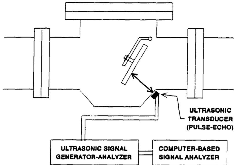
Figure 5 A simplified depiction of the ultrasonic monitoring method used by the CHECKMATE™II system available from ITI Movats, Inc.
