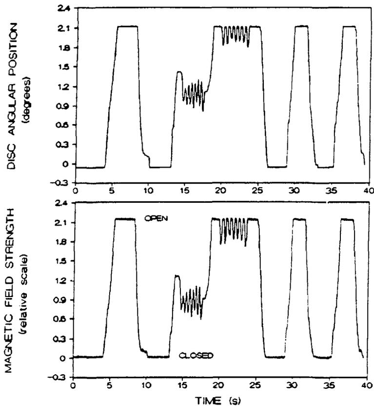
Figure 8 Comparison between magnetic field strength signals obtained with MFSA and disc angular position measurements (measured mechanically).
