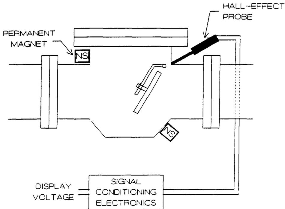
Figure 15 Simplified depiction of the external DC magnet check valve monitoring method developed by ORNL (note magnet polarities).
