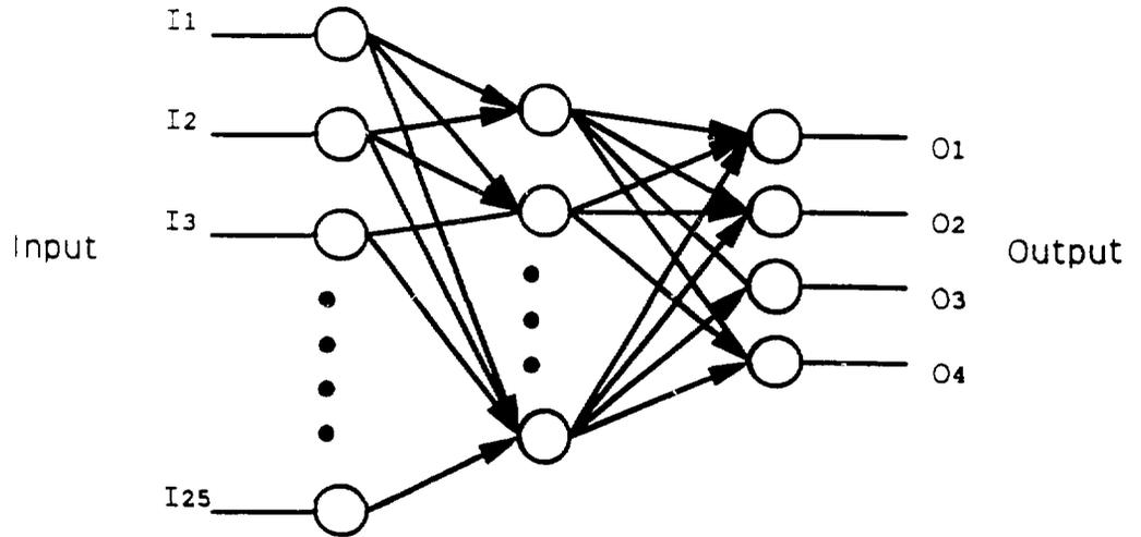
Fig. 1. Basic architecture of the backpropagation neural network used in the investigations.
