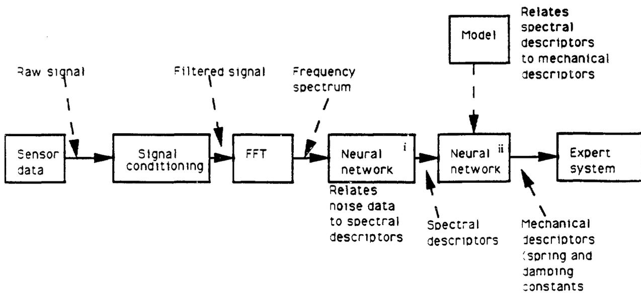
Fig. 6. Block diagram of a method for interpreting detector signal noise data using embedded neural networks.
