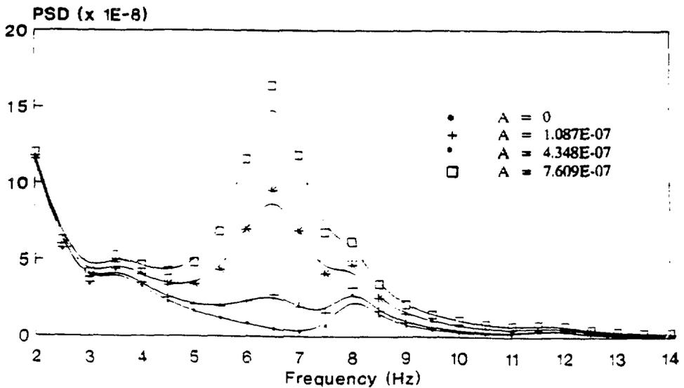
Fig. 4. Effect of variation in pole strength on power spectral density data.
