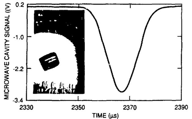
Fig. 4. Microwave cavity signal and photograph of a 3.4- × 4.3-mm pellet at 1.4 km/s.
