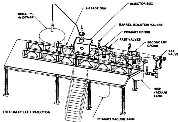
Fig. 1. Perspective view of the TPI installation on the TF-TR.
