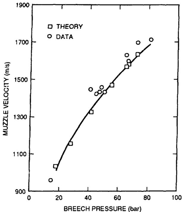
Fig. 5. Pellet speed vs breech pressure for gun 1.
