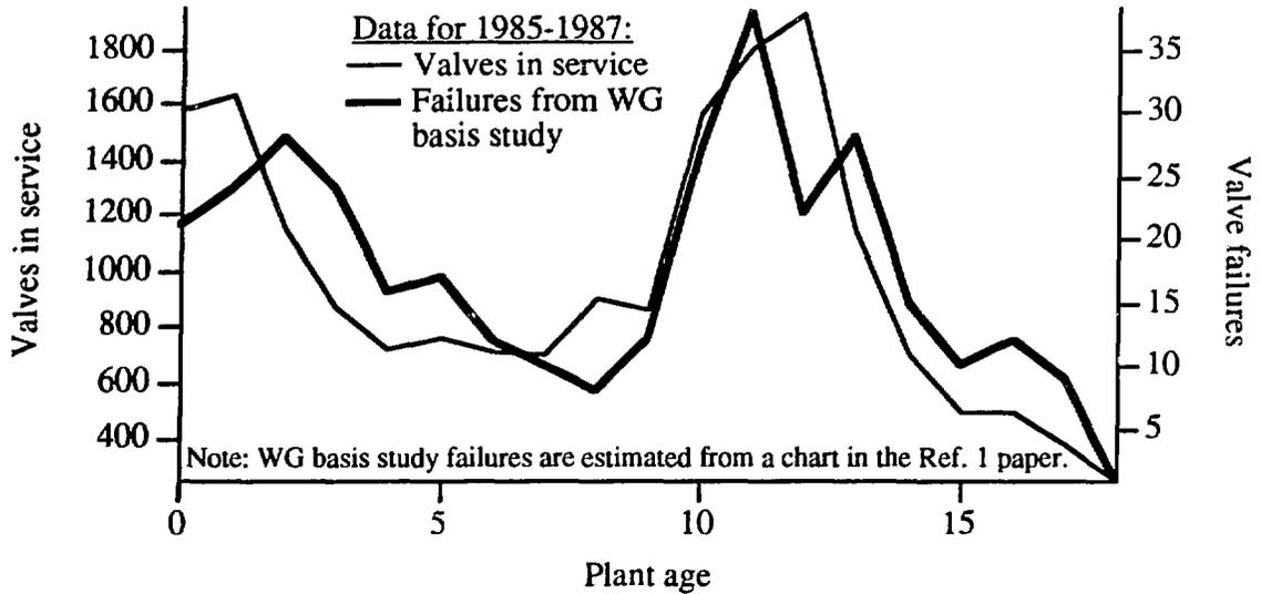
Figure 1. Comparison of Failures from Scott paper and Valves in Service
