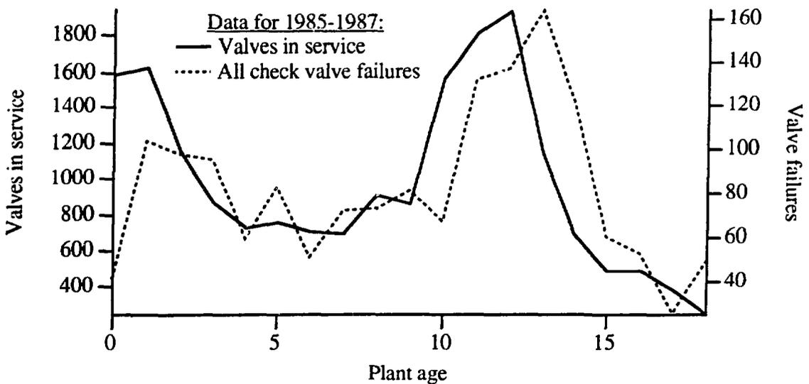
Figure 2. Comparison of All Check Valve Failures and Valves in Service
