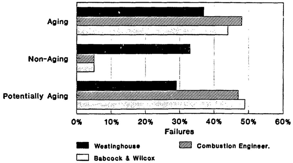
Figure 2. CRD system failures due to aging
