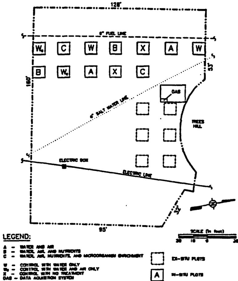
Figure 2. Test cell layout for bioremediation demonstration.
