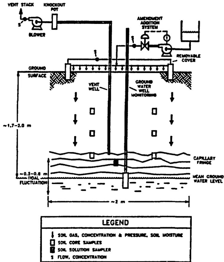
Figure 3. In situ test cell cross section.
