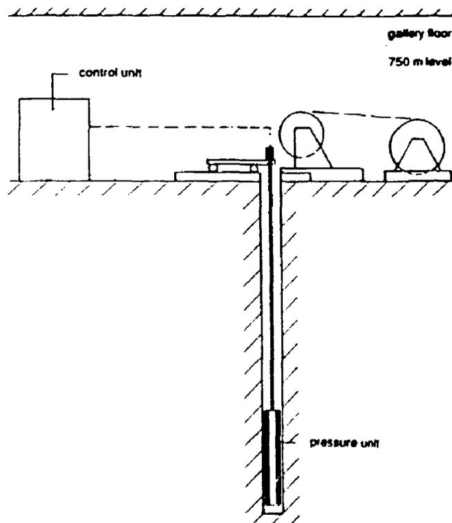
Fig. 1.1. Schematical setup of the Variable Pressure Device.
