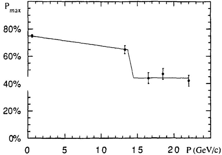
Figure 6: The maximum AGS beam polarization<sup>3</sup> as function of the beam momentum. The solid line shows the sharp polarization loss near 14 GeV/c.
