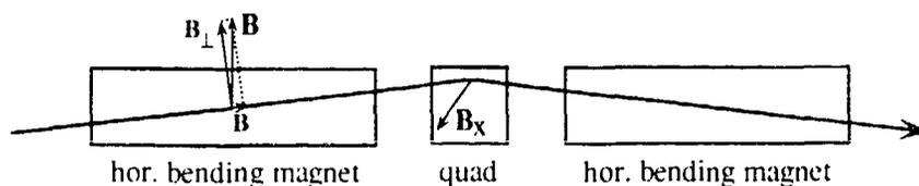
Figure 1: Fields along a trajectory oscillating in the vertical plane and passing through horizontally bending magnets and quadrupoles.
