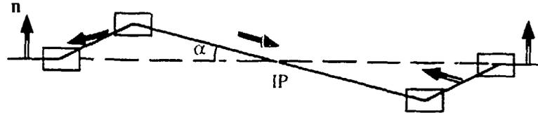
Figure 19: Schematic side view of an S-bend configuration of two spin rotators antisymmetric w.r.t. the collision point IP. Each rotator consists of two magnets vertically bending the electron trajectory by an angle  $\alpha$  and  $-2\alpha$  respectively. With  $\alpha = \pi/(2\gamma a)$  the spin closed solution  $\mathbf{n}$  is longitudinal at the IP.
