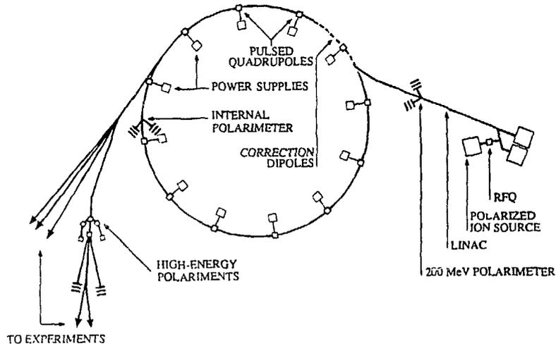
Figure 5: The AGS<sup>3</sup> lay-out for the acceleration of polarized protons.
