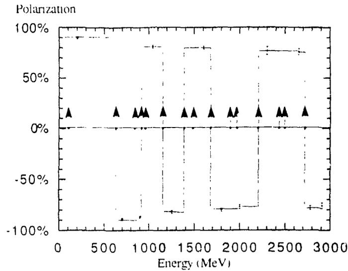
Figure 4: The vertical polarization as function of the proton energy during the acceleration cycle in Saturne<sup>1,2</sup>. The points with error bars are the experimental data. The arrows show the locations of the spin resonances. The solid line is a hand-drawn line showing the spin flips at the crossings of seven resonances.
