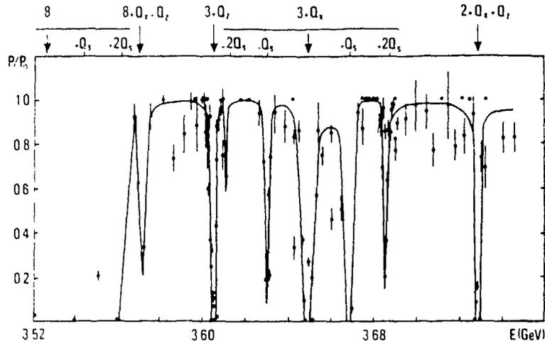
Figure 17: Relative polarization  $P/P_0$  ( $P_0 = 92.4\%$ ) versus beam energy at SPEAR<sup>39</sup>. The solid line is a hand-drawn line to guide the eye. The spin resonances labelled  $k + k_x Q_x + k_y Q_y + k_z Q_z$  are indicated above the figure.
