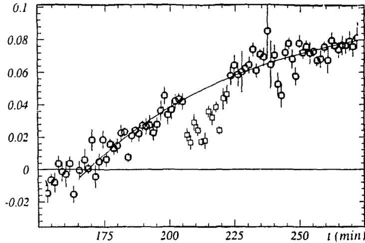
Figure 16: Polarimeter data versus time  $t$  at an energy of 46.55 GeV in LEP<sup>46</sup>. The fitted polarization time is 64 min leading to an equilibrium polarization of 20%.
