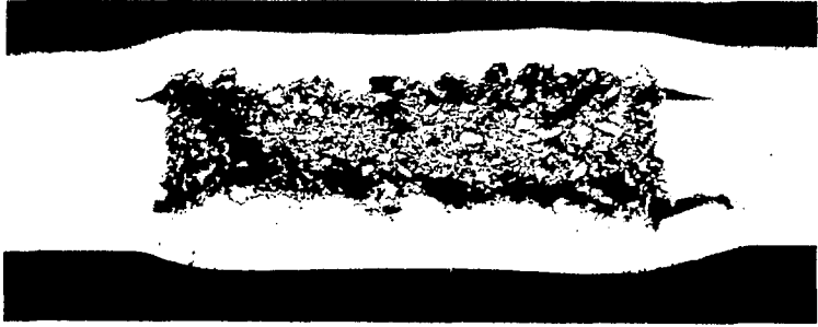
Fig.5 Cross-section of initially 1.38-mm-thick miniplate with fuel meat U_6(Fe_{0.6}Mn_{0.4})-Al after heating at 450°C for 120 h (see also Fig.4)
