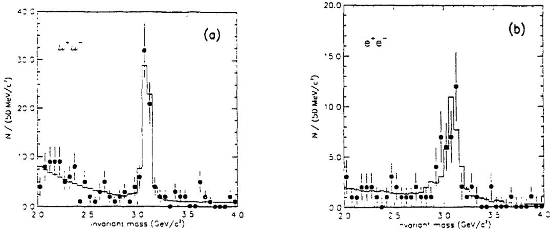
Figure 3: The  $J/\psi$  signal in the  $\mu^+\mu^-$  channel (Fig. 3a, 62  $J/\psi$  candidates) and in the  $e^+e^-$  channel (Fig. 3b, 38  $J/\psi$  candidates).
