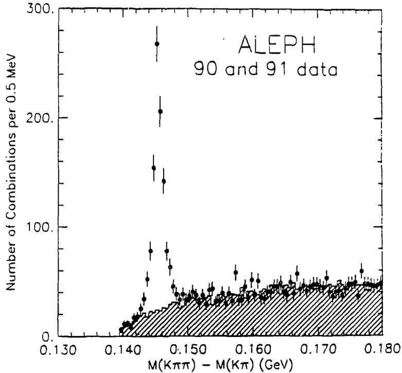
Figure 1:  $D^*$  signal: Mass difference distribution  $M(K \pi \pi) - M(K \pi)$  for  $x E(K \pi \pi) > 0.25$ . The  $k\pi$  invariant mass is required to be between 1.835 and 1.895  $GeV/c^2$  ( $D^0$  mass region). The hatched area is the combinatorial background.
