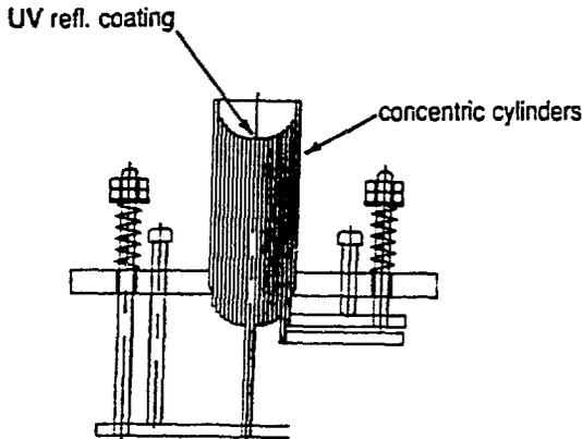
Figure 2: Laser pulse shaping reflector
