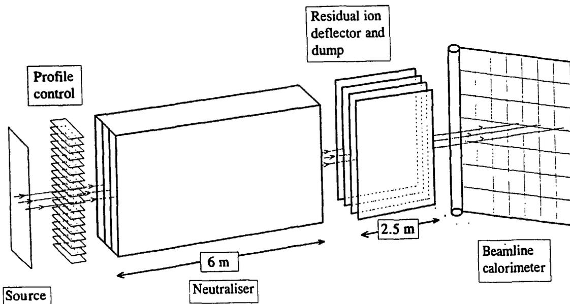
**FIGURE 6: SCHEME OF THE NEW BEAMLINE DESIGN**
