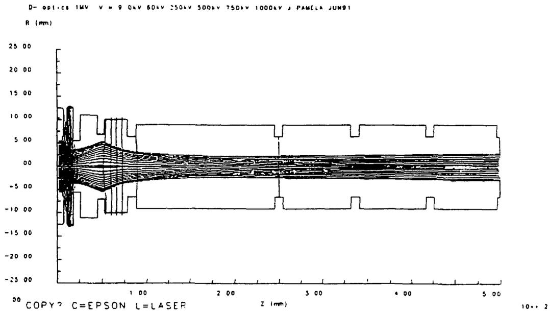
**FIGURE 4: 1.3 MV, 16 mA/cm<sup>2</sup> (ACCELERATED) D- BEAMLET OPTICS CALCULATION**
