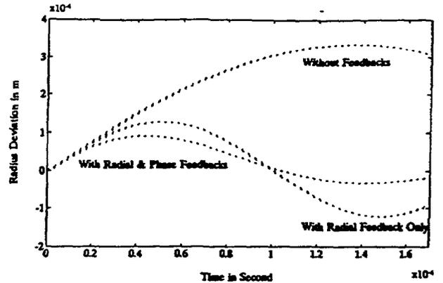
Figure 3. Beam radial deviation under various feedback conditions.
