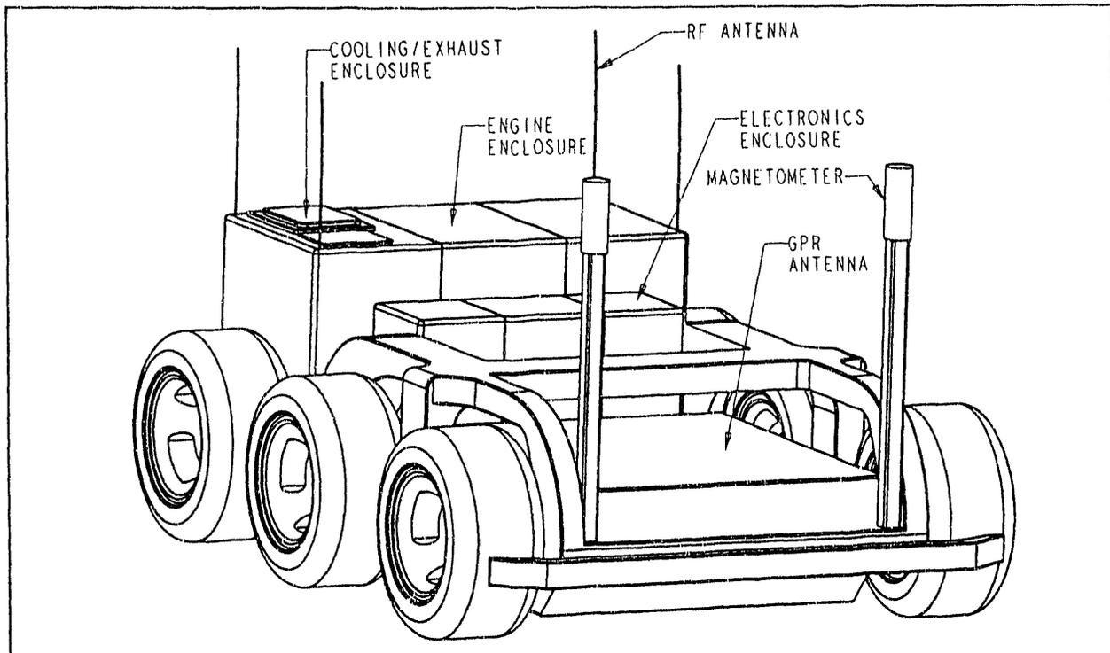
Figure 2. A drawing of the low-signature survey vehicle.
