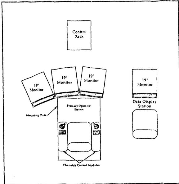
Figure 3. Layout of the high-level control station.
