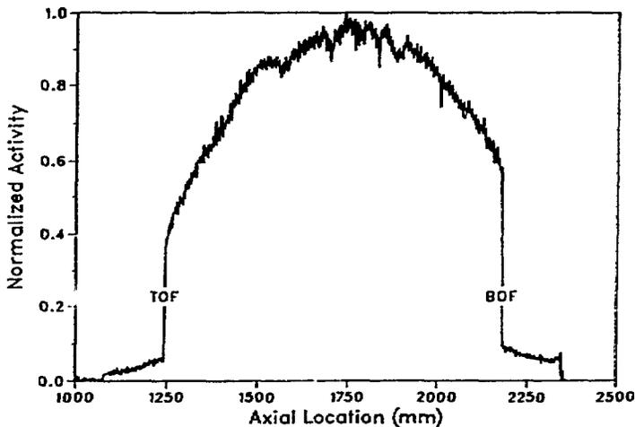
Because of the fuel column elongation, the top end of the fuel was raised above the core where the fission densities were markedly lower.
