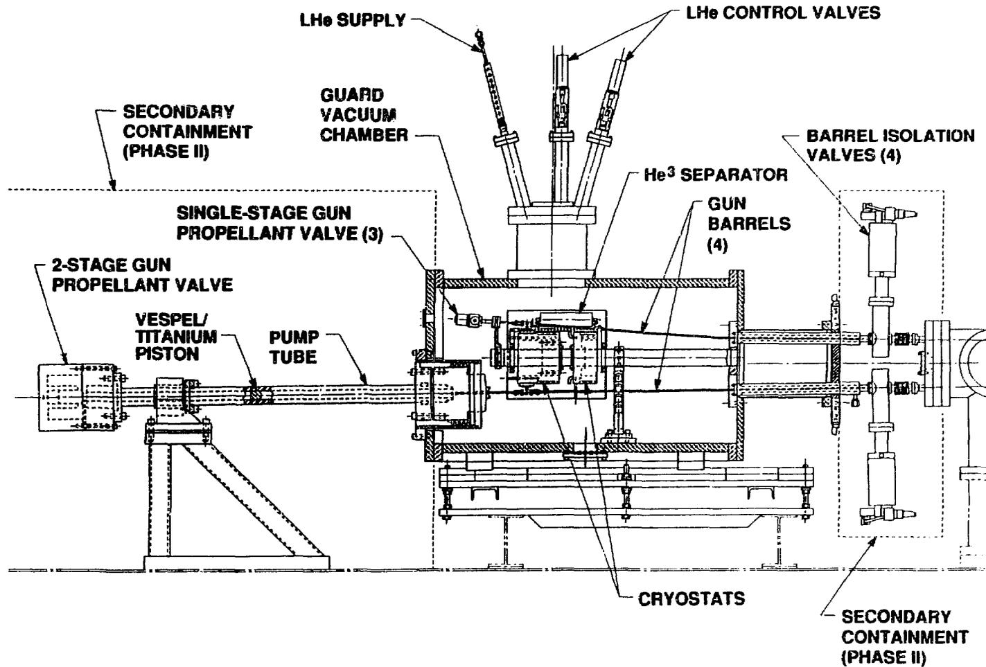
Fig. 2. The TPI injector and two-stage light gas gun assembly.
