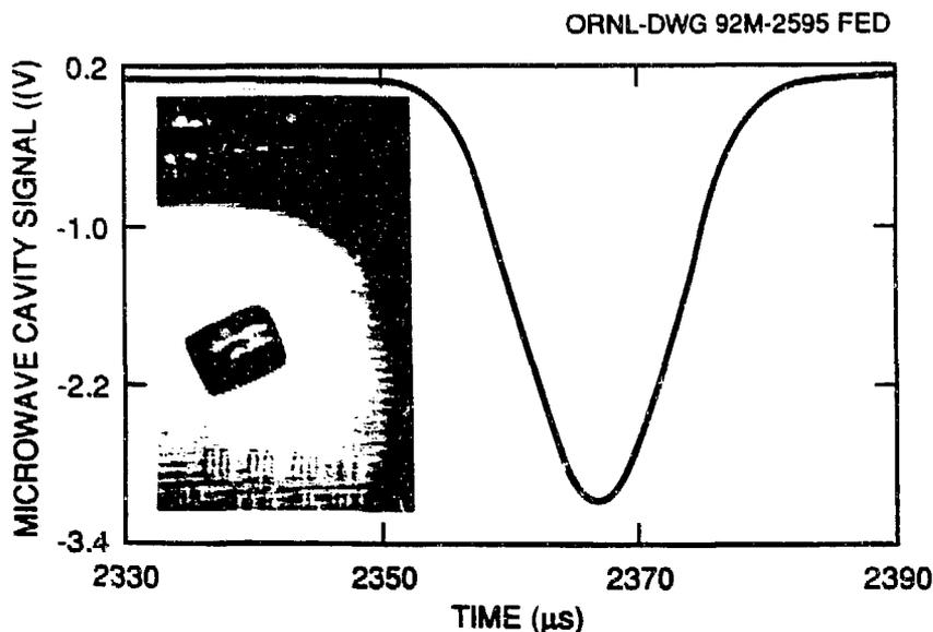
Fig. 5. Microwave cavity signal and photograph of a 3.4- by 4.3-mm pellet at 1.4 km/s.
