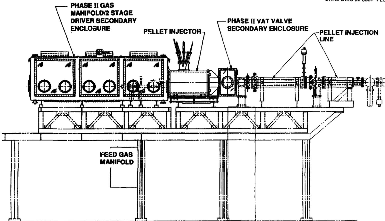
Fig. 4. The TPI secondary containment system for operation with tritium pellets.
