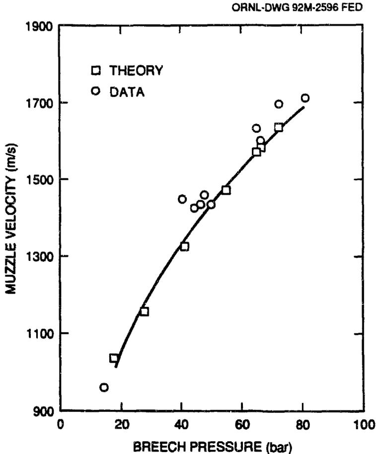
Fig. 6. Pellet speed vs breech pressure for gun 1.
