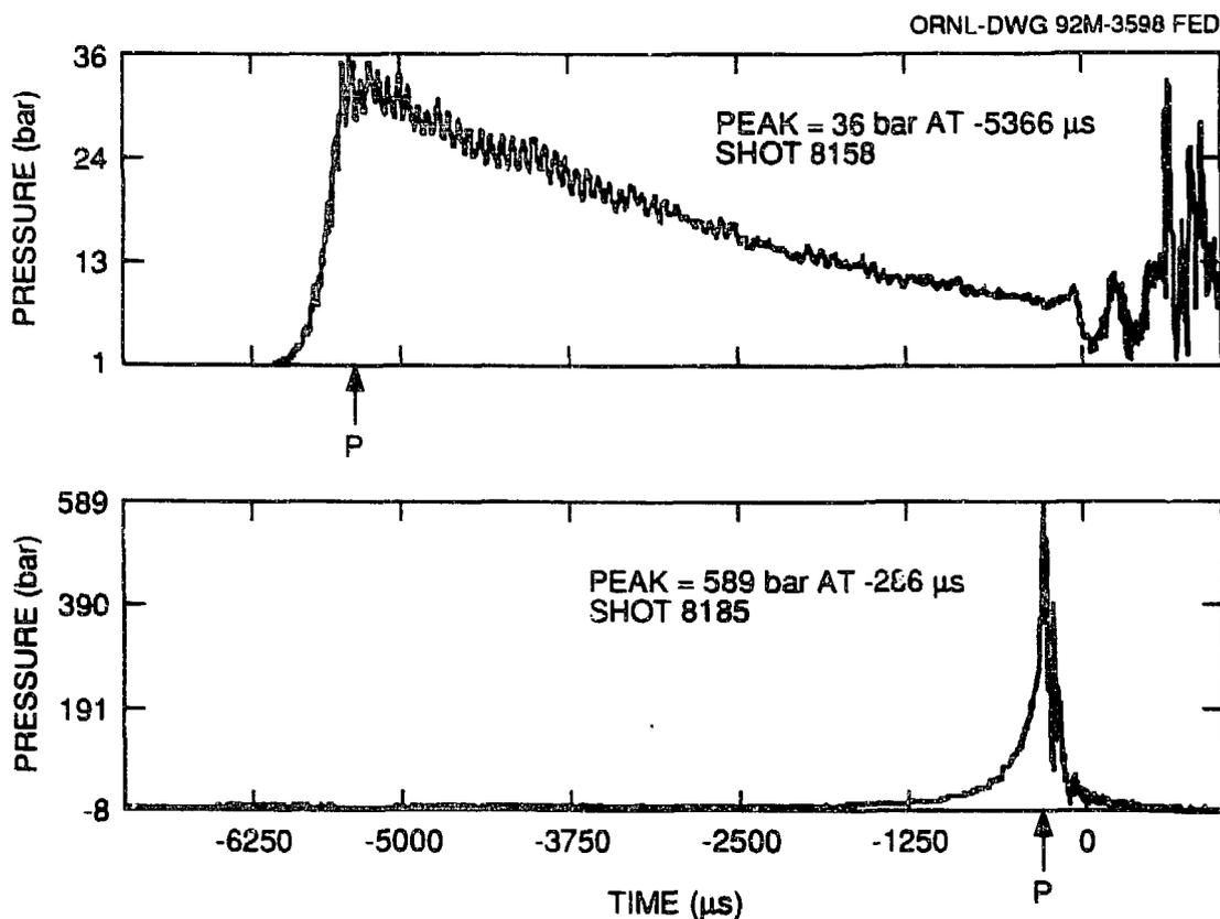
Fig. 7. Data from a 2.8 km/s deuterium pellet shot (gun 4). Upper plot is pressure in breech end of pumptube and lower plot is pressure in the two-stage driver high pressure head.
