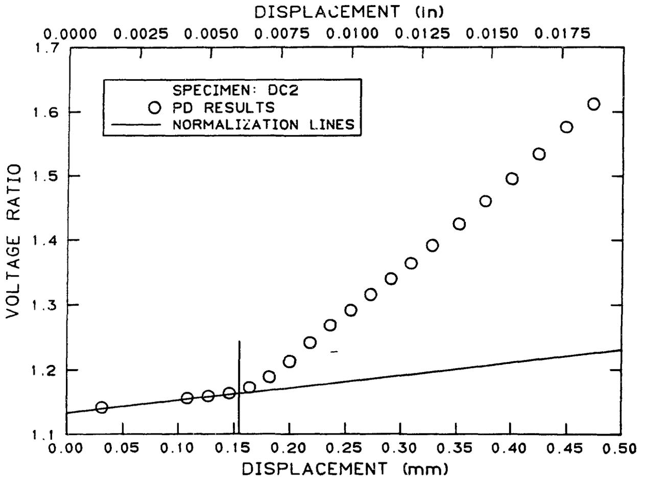
Fig. 7. A plot of the voltage ratio versus the load line displacement for one of the disk compact specimens. The straight line is used to assist the selection of the point of initial deviation from linearity. The vertical line shows the point selected as the beginning of crack extension.
