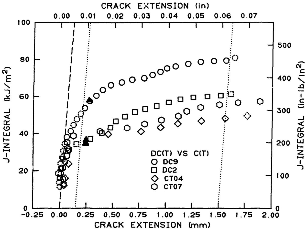
Fig. 10. A comparison between the J-R curves obtained by unloading compliance from 1/2 T compact specimens and the 0.18 T disk compact specimens. The compact specimens gave similar  $J_{Ic}$  values, but the J-R curves had lower slopes (lower tearing moduli).
