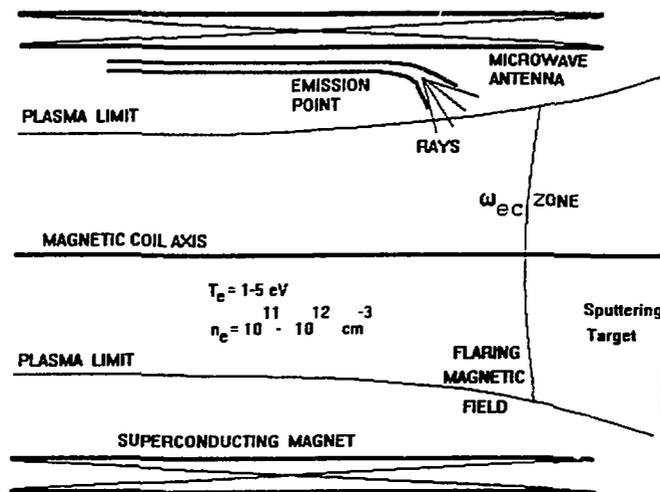
Fig. 1. Scheme of the ECR source in a flaring magnetic field.
