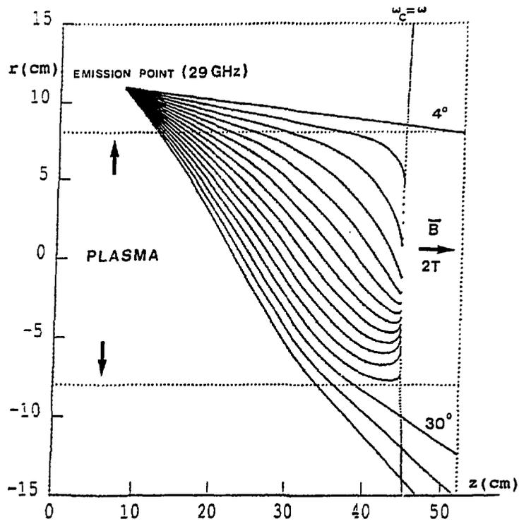
Fig. 2. Ray tracing at 29 GHz for the emission angles between  $4^\circ$  and  $34^\circ$ . Here,  $B = 2T$ ,  $n_e = 10^{12} \text{ cm}^{-3}$  and  $T_e = 5 \text{ eV}$ .
