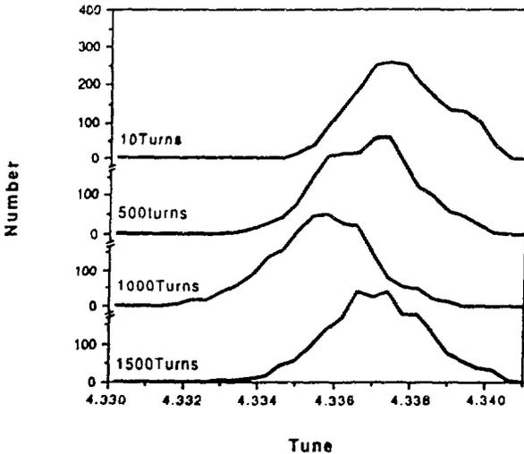
Fig. 3. Horizontal tune distribution of circulating beam. The horizontal tune value shifts to the resonance by the acceleration. Eight percent of the circular particle are extracted immediately after 1000turns and the tune goes away from the resonance by the relaxation of the space charge.
