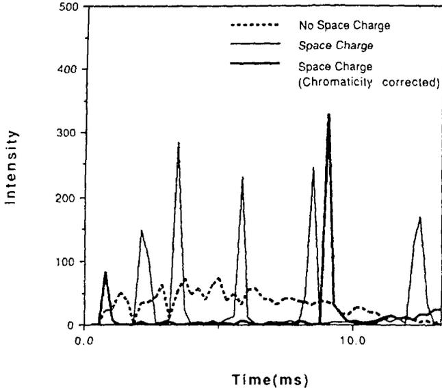
Fig.2. Calculated time structures of the beam spill. Dashed, dotted and solid lines mean the no space charge case, the case satisfies the overlapping condition and includes the space charge, and the case includes the space charge and has a large chromaticity, respectively.
