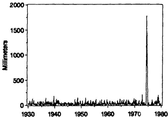
Figure 2. Plot of monthly precipitation totals through time for a station with a "gross" data processing error.
