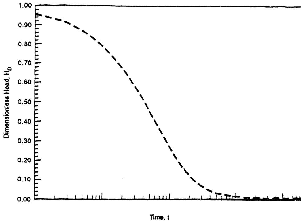
Figure 1 - Typical single-well slug test.
