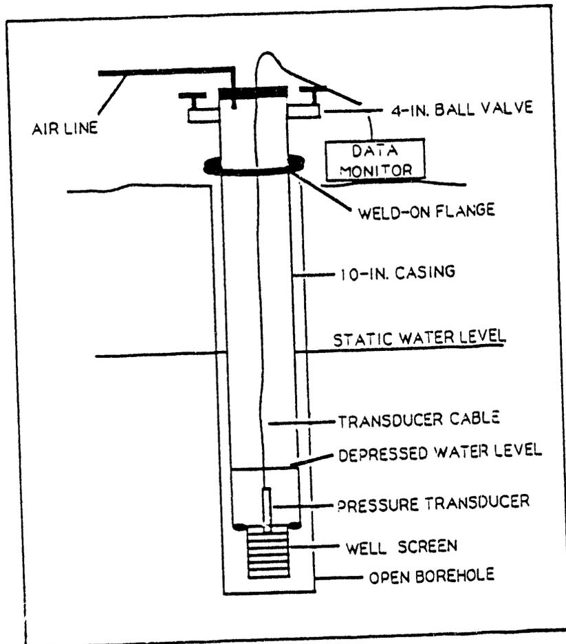
Figure 6 - Borehole configuration and test equipment for the stress well.
