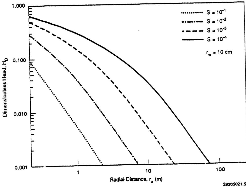
Figure 4 - Predicted maximum slug interference test response as a function of distance.
