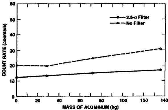
Fig. 7. Coincidence count rate as a function of aluminum matrix mass for the filtered ( $2.5\sigma$ ) and unfiltered cases.
