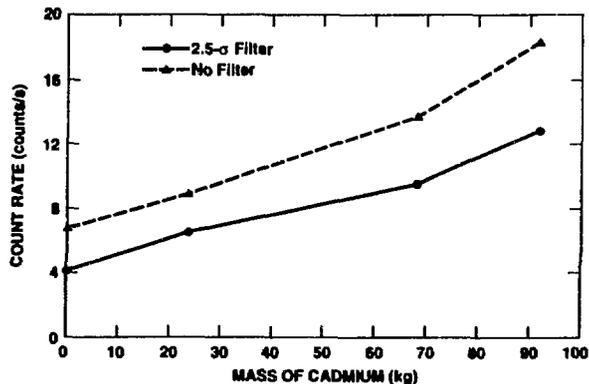
Fig. 9. Coincidence count rate as a function of cadmium matrix mass for the filtered ( $2.5\sigma$ ) and unfiltered cases.
