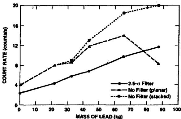
Fig. 10. Coincidence count rate as a function of lead matrix mass for the filtered ( $2.5\sigma$ ) and unfiltered cases.
