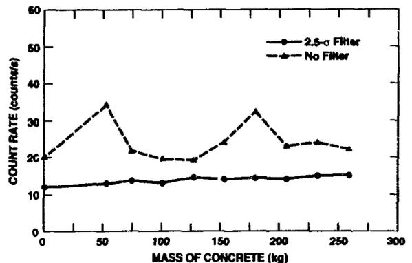
Fig. 6. Coincidence count rate as a function of concrete matrix mass for the filtered ( $2.5\sigma$ ) and unfiltered cases.
