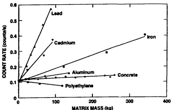
Fig. 11. Filtered (2.5  $\sigma$ ) coincidence count rates for each matrix.
