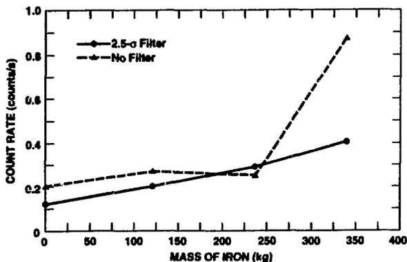
Fig. 8. Coincidence count rate as a function of iron matrix mass for the filtered ( $2.5\sigma$ ) and unfiltered cases.
