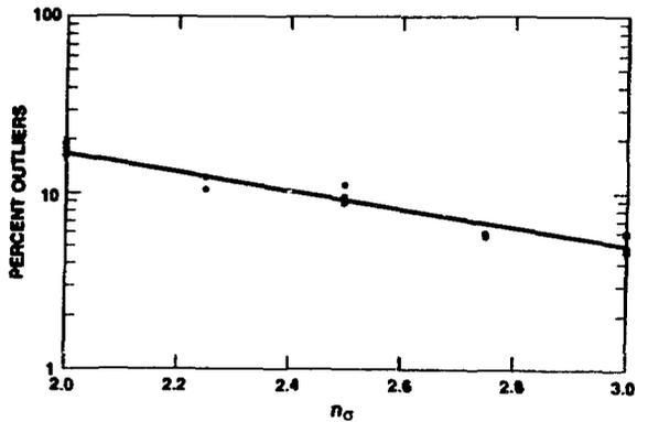
Fig. 3. Run-rejection percentage with an empty 200-ℓ drum placed in the counter.
