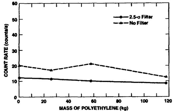
Fig. 5. Coincidence count rate as a function of polyethylene matrix mass for the filtered ( $2.5\sigma$ ) and unfiltered cases.
