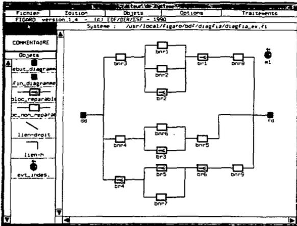
Fig. 1 : Graphic data acquisition for a reliability diagram
