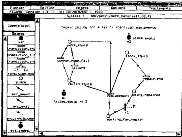
Fig. 2 : Graphic data acquisition for a Petri net
