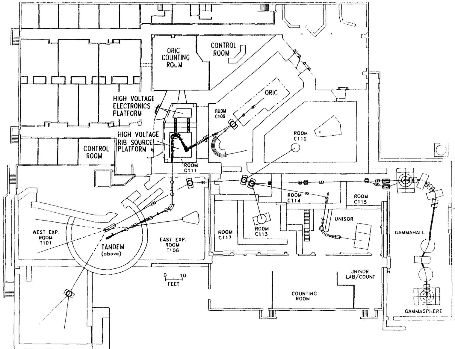
Figure 1. FLOOR PLAN OF THE HHIRF SHOWING THE NEW RIB PLATFORM AND ASSOCIATED BEAM LINES. ALSO SHOWN IS THE PLANNED GAMMAHALL ADDITION.
