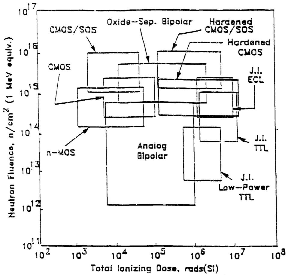
Fig. 2. Schematic representation of microcircuit susceptibility.<sup>3</sup>
