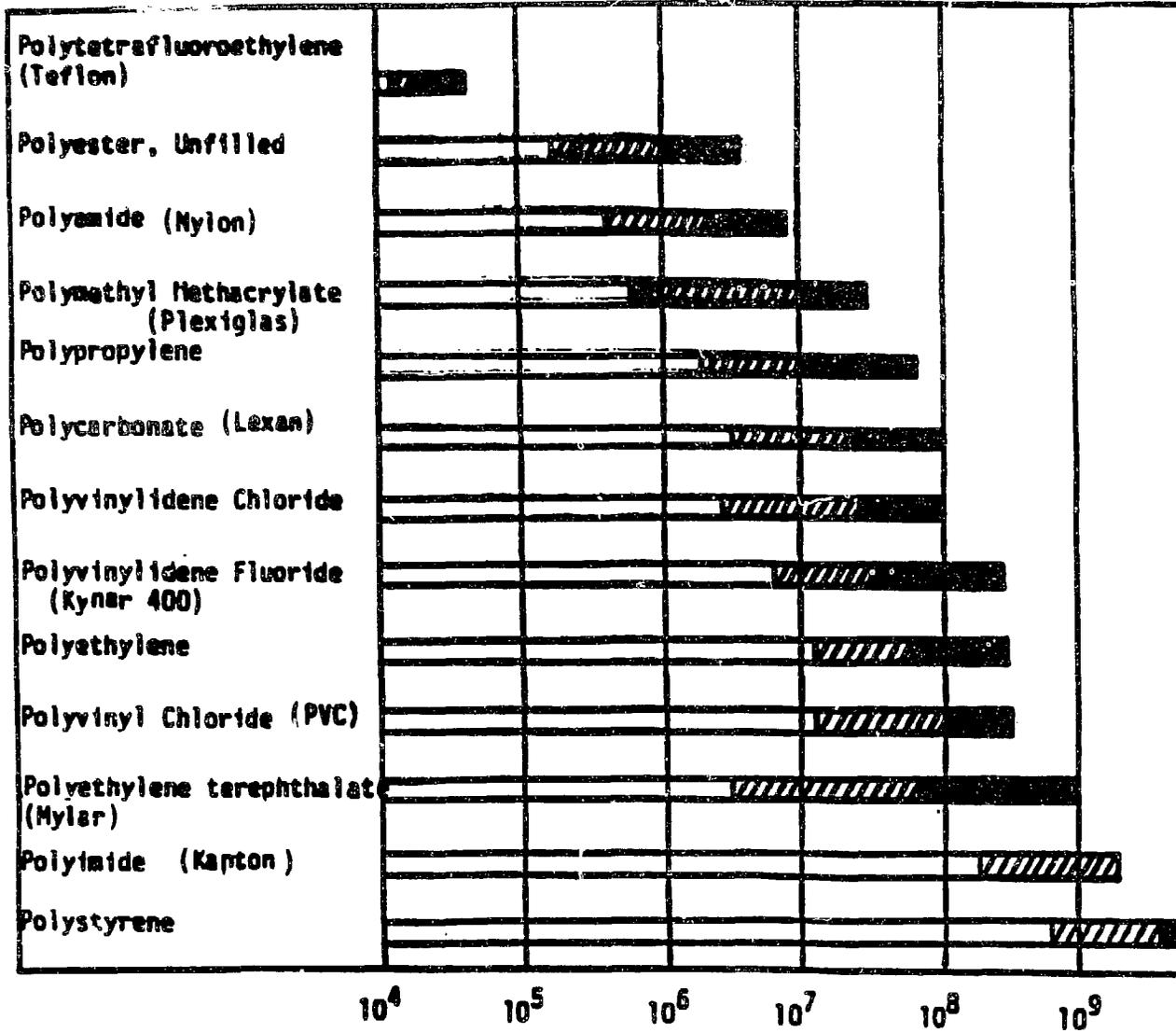
Fig. 3. Radiation effects on polymer dielectrics.<sup>4</sup>
