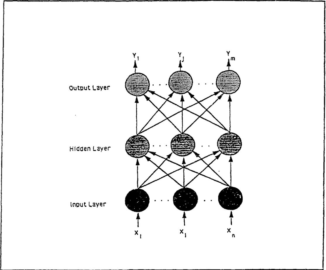
**Figure 3. Three-layer Neural Network Architecture.**
