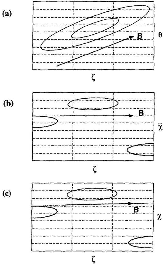
Fig. 1. Grid (dashed lines), magnetic field (arrows), and turbulent structures (ellipses) at a single radial location, as seen in (a) toroidal-poloidal coordinates, (b) ballooning coordinates, and (c) quasibalooning coordinates.
