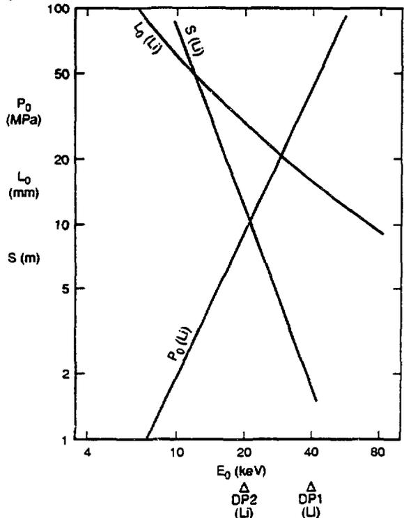
Fig. 7. Projected 10-km/s electron-beam rocket accelerator parameters for lithium pellets and beam perveance =  $12 \mu\text{P}$ .
