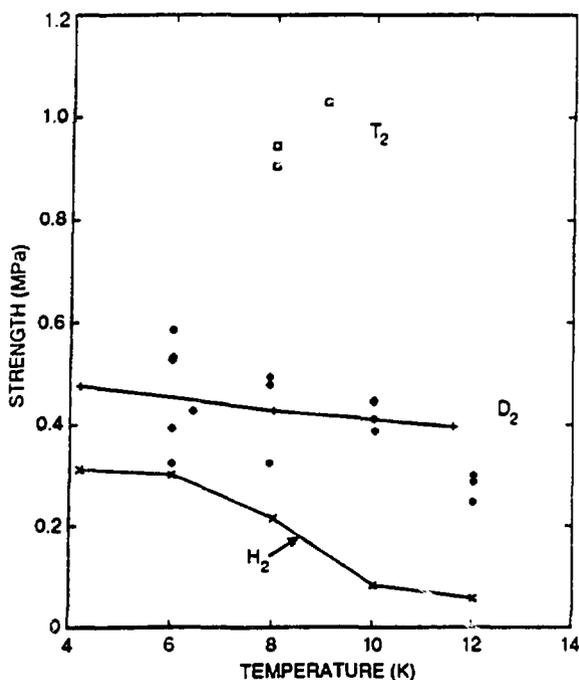
Fig. 4. Measurements of the shear strength of solid tritium.
