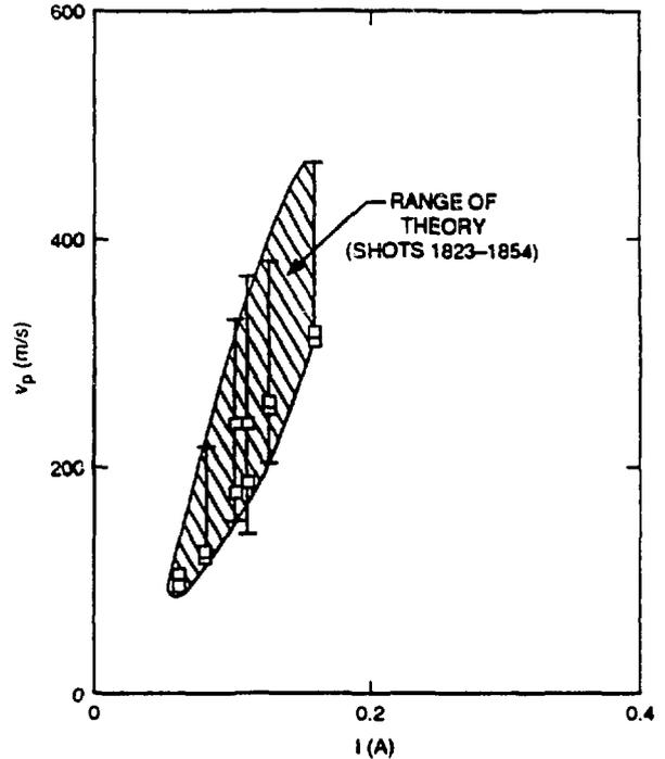
Fig. 6. Proof-of-principle electron-beam rocket accelerator performance.
