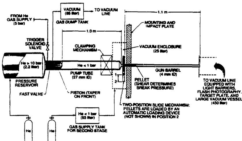
Fig. 5. Repeating two-stage light gas gun.
