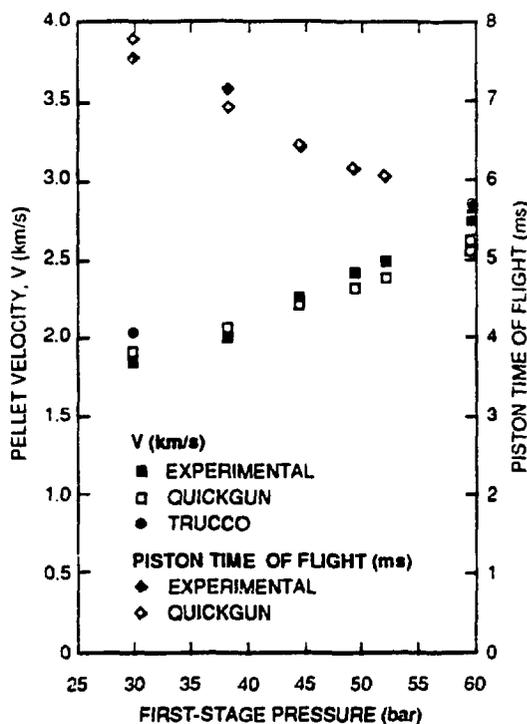
Fig. 3. TPI two-stage gas gun performance measurements and calculations.
