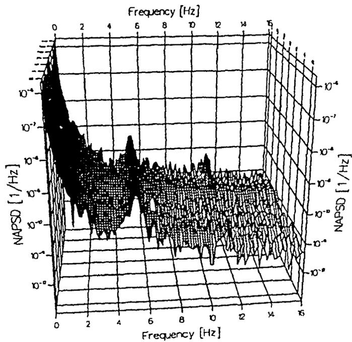
Fig. 11: NAPSD function versus time for Ex-Core Neutron Detector B in Experiment IRI12A.
