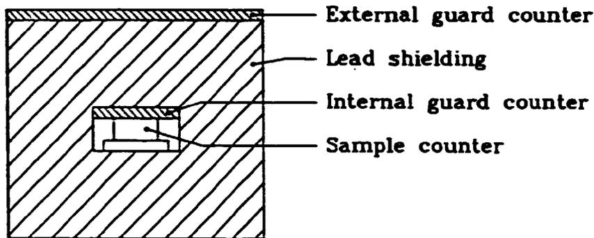
Fig. 2.3. Schematic diagram of the beta multicounter set-up with external guard counter.
