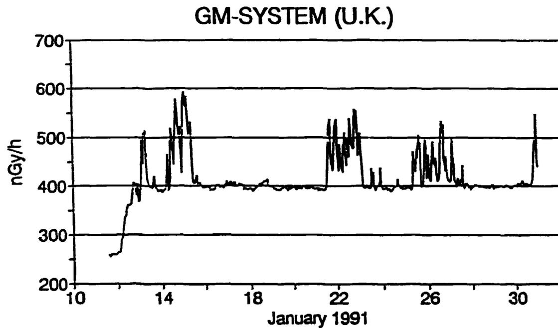
*Fig. 2.4. The air kerma rate variations at the Hinkley Point Power Station in January 1991 as measured by a Reuter Stokes high-pressure ionisation chamber (RS-system) and a GEC GM counter (GM-system).*
