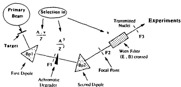
Fig. 2: Schematic view of a spectrometer composed with three selections (magnetic, energy-loss, velocity).
