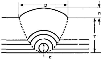
Fig. 2. Geometry of an ideal nodule defect in a multilayer stack. The surface diameter,  $D$ , is given by Eqn. 2.
