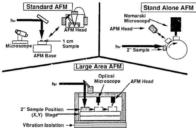
Fig. 1. Schematic representations of the AFM systems used for in-situ laser damage experiments.
