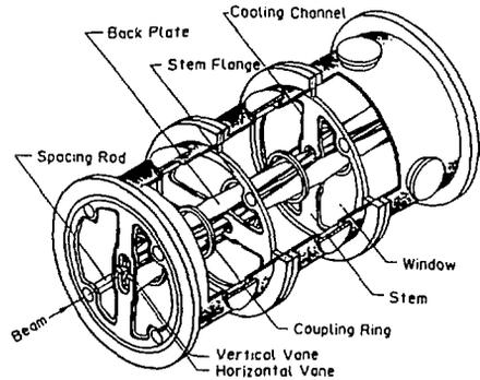
Fig.2 Structure of the prototype SCRfQ.
