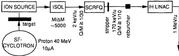
Fig. 1 Layout of the prototype facility at INS.
