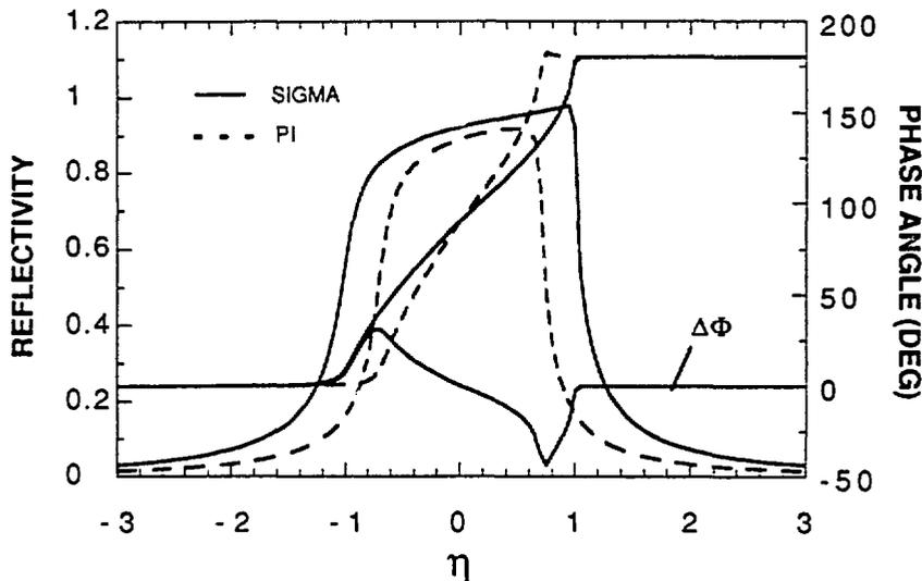
FIG. 5. Reflectivity, phase angle, and phase angle difference as a function of  $\eta$  (the scaled angle variable) for the  $\sigma$  and  $\pi$  components of the (220) reflection in Ge at 8 KeV. Because the phase difference is less than  $90^\circ$  per reflection multiple reflections are required to accumulate a total phase shift of  $90^\circ$  between the  $\sigma$  and  $\pi$  components. (With permission from B.W. Batterman, to be published).
