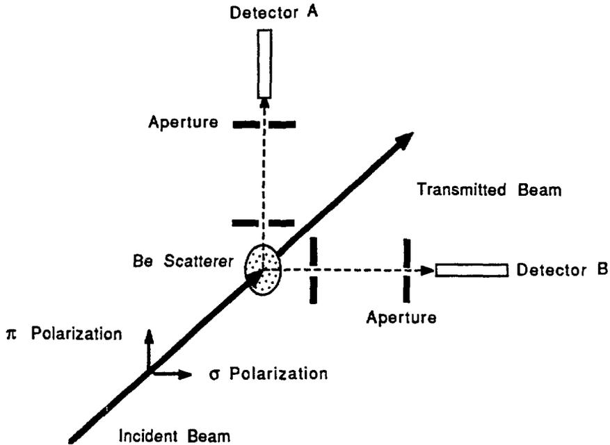
FIG. 1. Schematic of a Compton polarimeter for linear polarization analysis. The incoming beam, scattered by thin foil of Be, is detected by two detectors oriented at right angles to each other and to the beam. Apertures define the angular acceptance of the detectors. Detector A is sensitive to  $\sigma$  polarized x-rays while Detector B is sensitive to  $\pi$  polarized x-rays.
