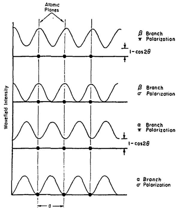
crystal, while the  $\beta$  wavefields have a greater interaction with the crystal than an arbitrarily oriented wavefield. Put in a more qualitative way, when the crystal is isotropic, all wavefields in the crystal have the same wavevector given by (following the notation of Hart [3]):
