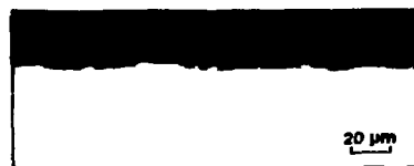
Cross-section micrography after 500-hour Pt coupling in 14.4N \text{HNO}_3
