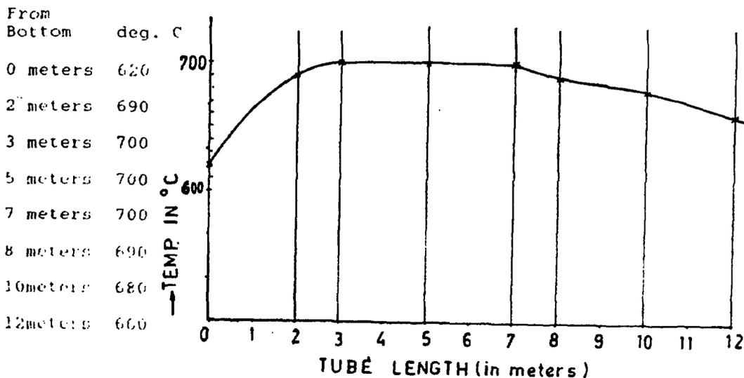
**Skin temperatre profile of cracker tube outer wall**
