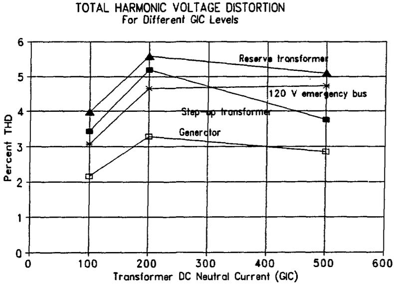
**Figure 7.** Comparison of THD for different GIC levels.
