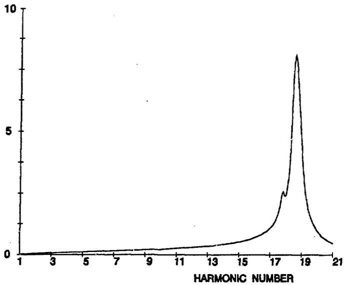
**Figure 16.** Transmission line impedance function for normal station configuration and nominal system parameters.
