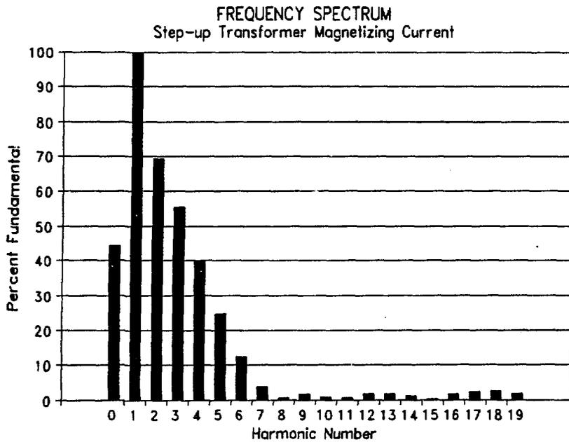
**Fig. 3.** Frequency spectrum of generator step-up transformer magnetizing current.
