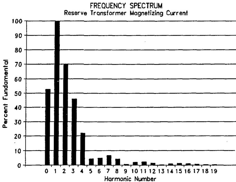
**Figure 9.** Frequency spectrum of the magnetizing current in the reserve station service transformer, with separate 115 kV line.
