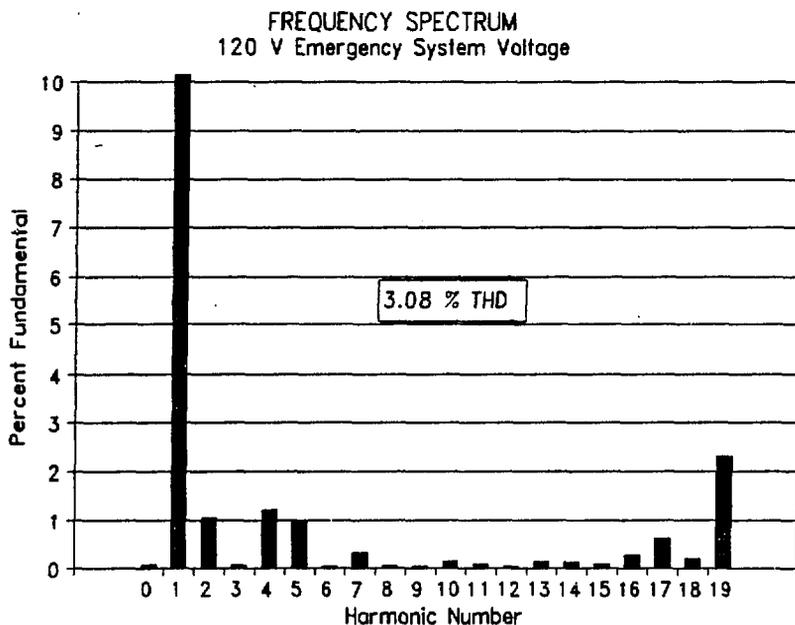
**Figure 5.** Frequency spectrum of 120 V emergency system voltage.
