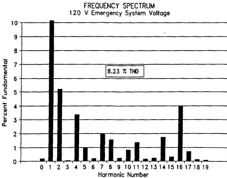
Figure 13. Frequency spectrum of 120 V emergency system voltage, with separate 115 kV line to reserve station service transformer.
