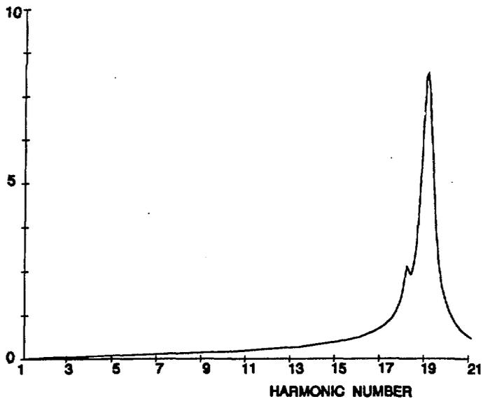
**Figure 19.** Transmission line impedance function for normal station configuration with 49.07 mile line.
