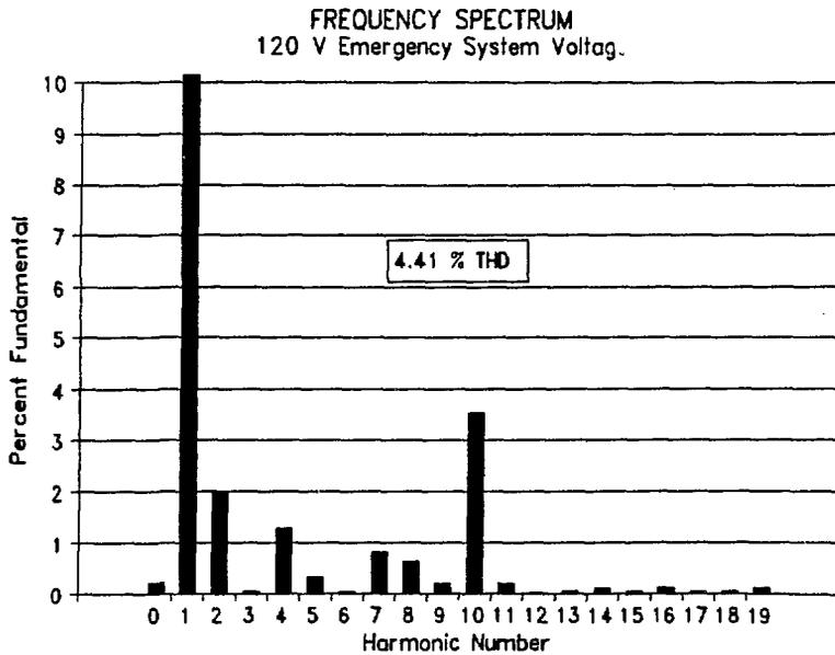
**Figure 15.** Frequency spectrum of 120 V emergency system voltage, during start-up mode.
