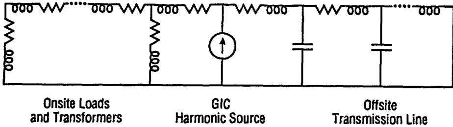
**Figure 6.** Simple model for distribution of GIC-induced harmonics between power station and transmission system.
