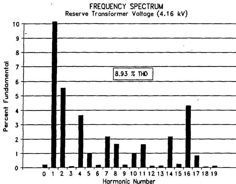
**Figure 11.** Frequency spectrum of A-phase reserve station service transformer voltage on 4.16 kV side, with separate 115 kV line.
