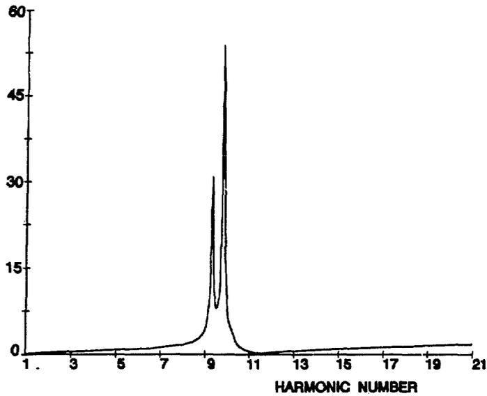
**Figure 18.** Transmission line impedance function for station start-up mode with nominal system parameters.
