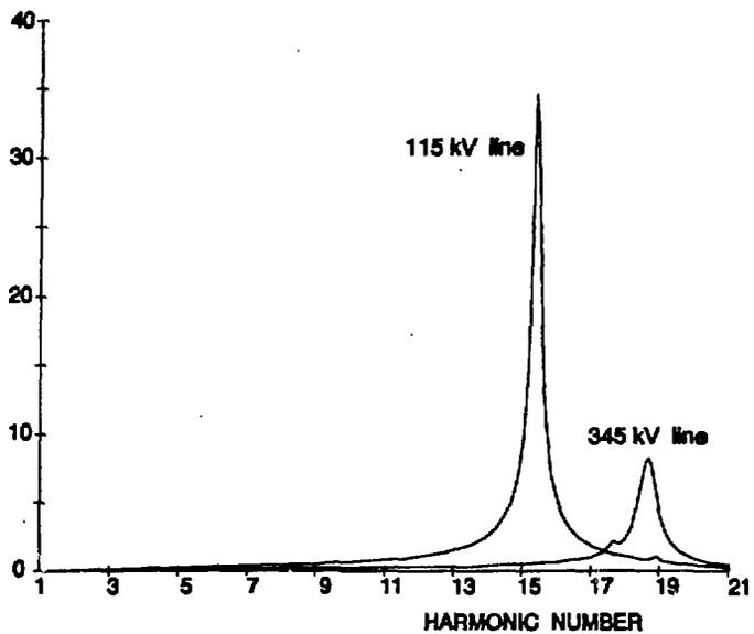
**Figure 17.** Transmission line impedance functions for station with separate 115 kV service and nominal system parameters.
