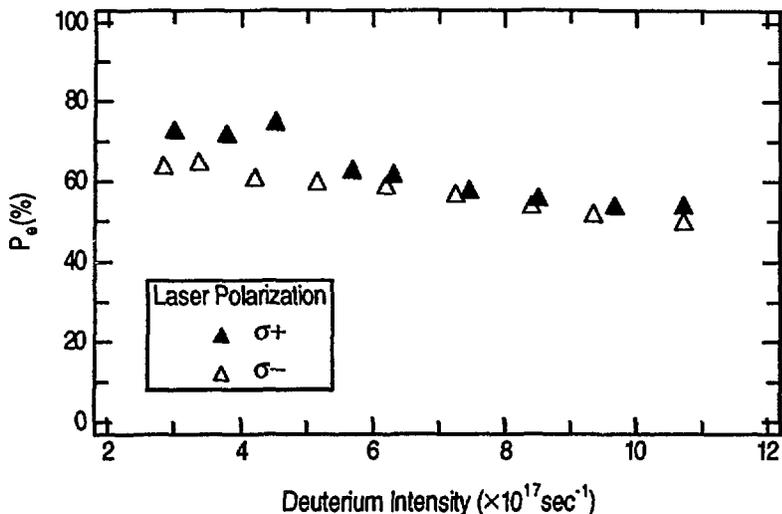
Figure 2. Deuterium polarization as a function of total deuterium intensity for both orientations of laser polarization.
