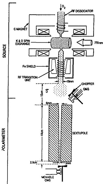
Figure 1. Schematic diagram of the polarized source and polarimeter.
