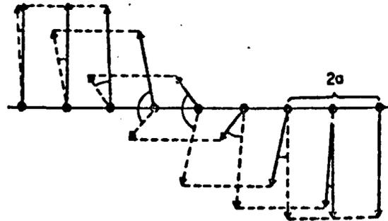
Fig. 2 Walls:  $H_1$  displaces the walls and  $M$  turns, creating large transverse hf fields.
