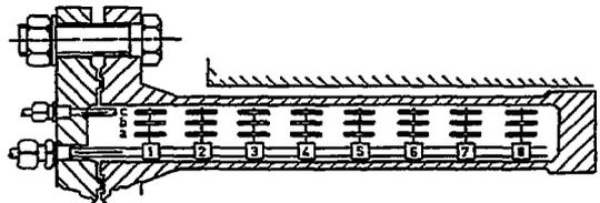
Figure 1: Laboratory autoclave with test samples (numbers indicate the stack, letters the stack position)
