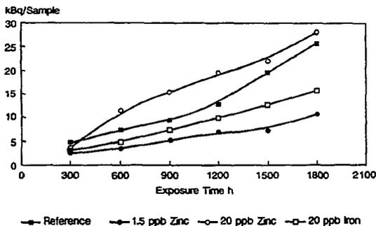
Figure 2: Co-58 activity measured on steel samples in stack 5, position (a), after different exposure times (test conditions as described in Table 4)
